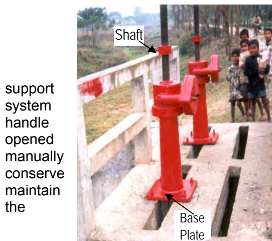
Figure-13 Raising of Vertical Gate
