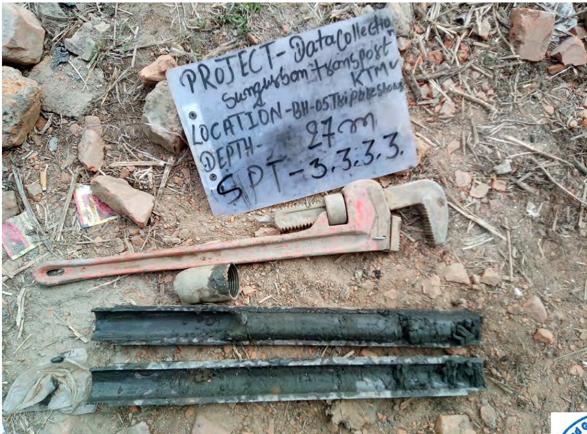
Retrieving Soil Samples through SPT Tubes
