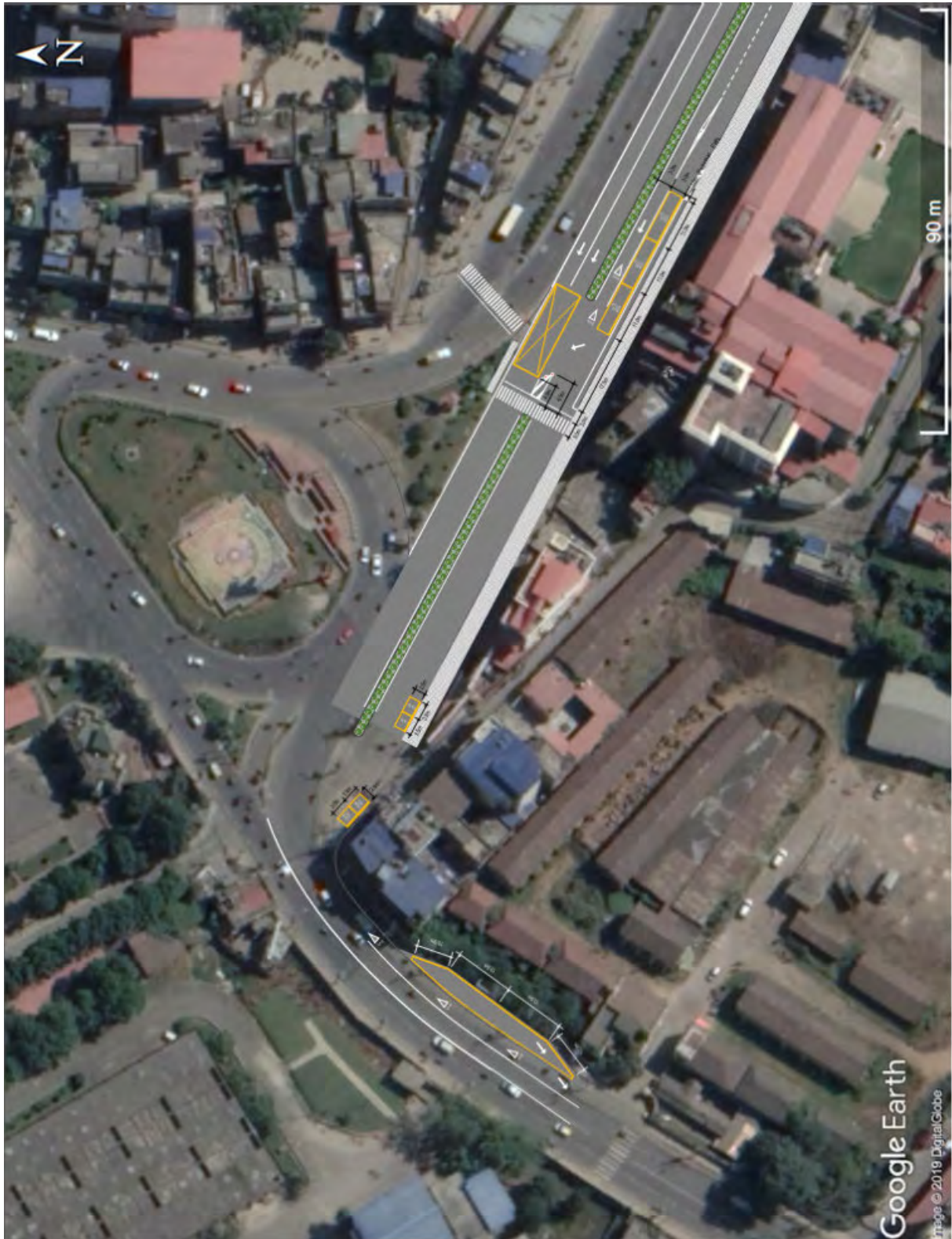
Figure 5.1.2 Road Marking Plan for Pilot Project at Maitighar Intersection
