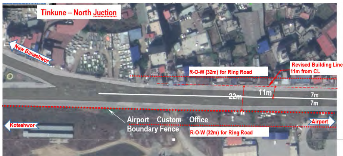
Figure 4.6.6 Detailed ROW of Tinkune Intersection
