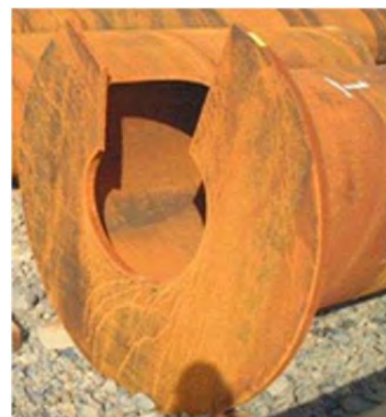
Tip of the Rotary Penetration Steel Pile
