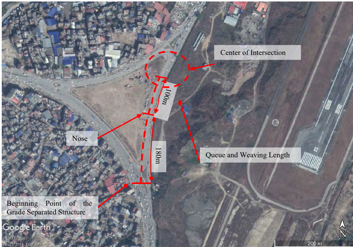
Figure 4.4.5 Plan View of Tinkune Intersection with Option 2 Applied
