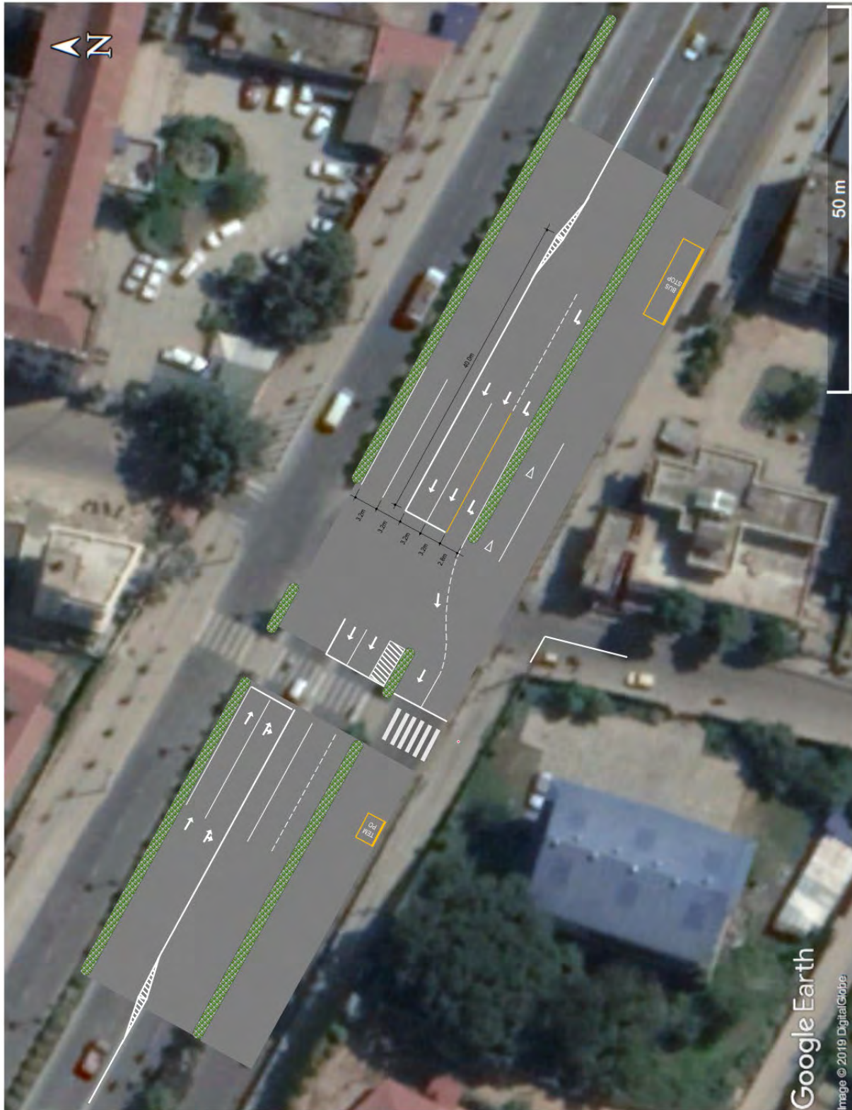
Figure 5.1.3 Road Marking Plan for Pilot Project at Babar Mahal
