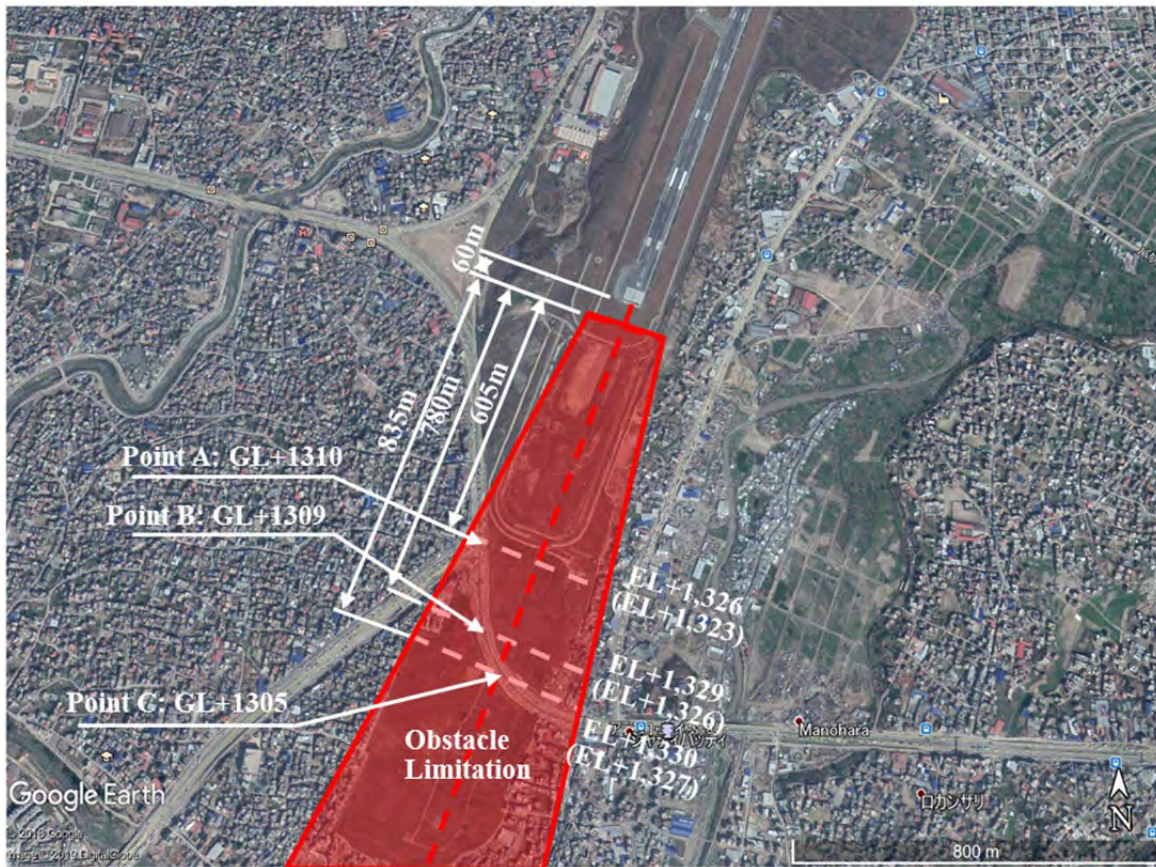
Figure 4.4.7 Plan View of Obstacle Limitation
