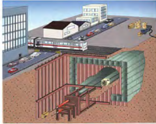
Figure 4.5.10 Element Jacking Method
