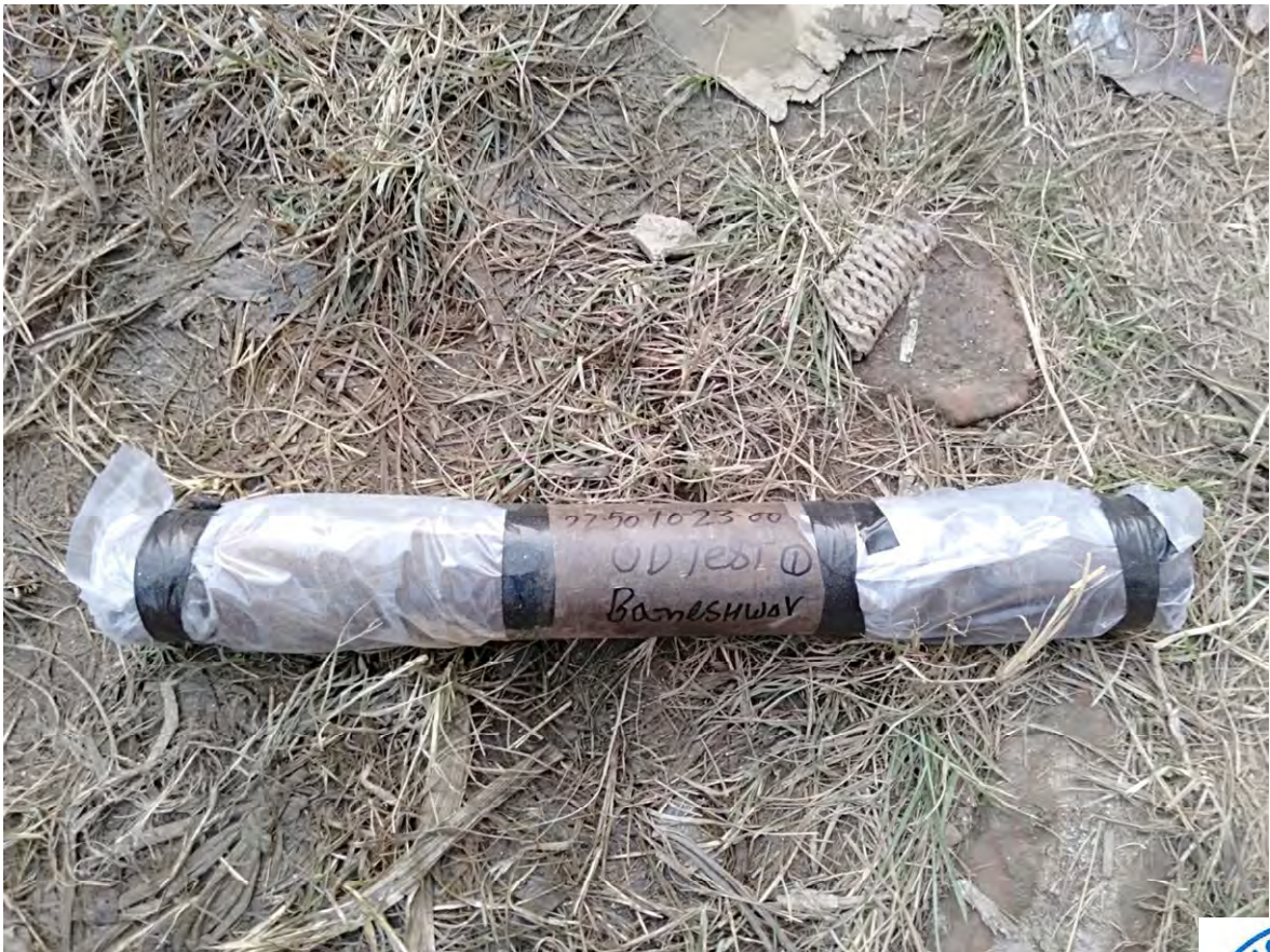
Preserving UD Samples in a UD Samplers
