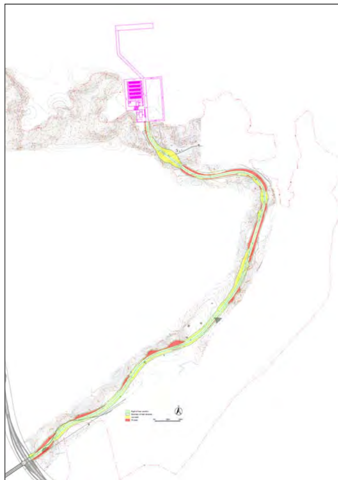
Figure 11.3.14 Cut and Fill Areas along the SEZ Main Road (Yellow: Cutting Area, Red: Filling Area)
