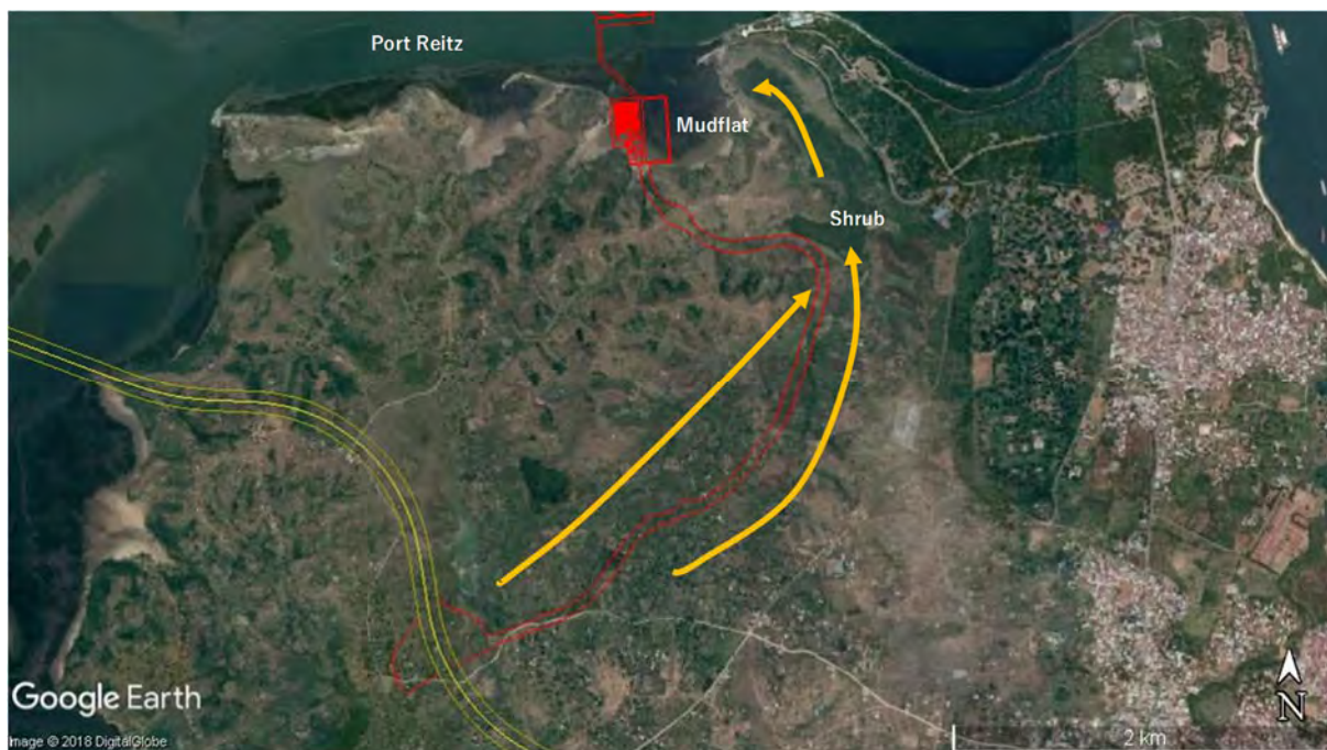
Figure 11.3.31 Drainage Route of Rainwater Runoff around SEZ Main Road
