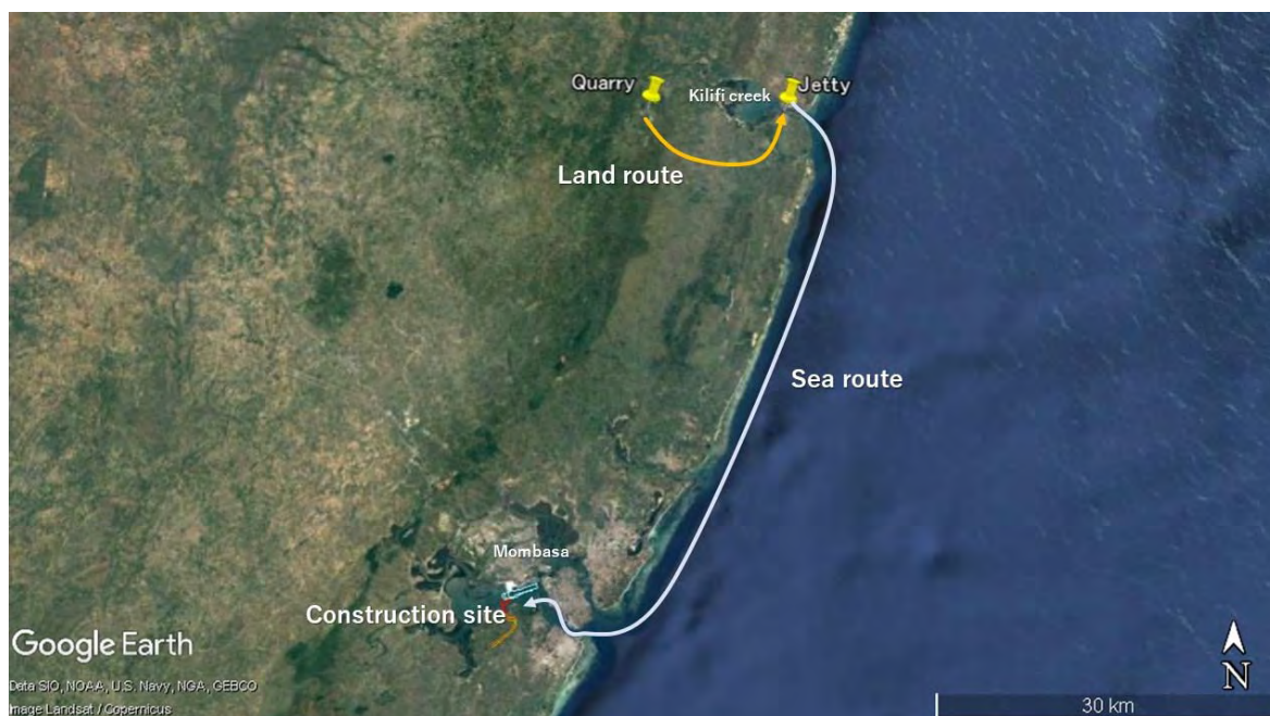
Figure 11.3.12 Planned Route of Material Transportation from Quarry to Construction Site
