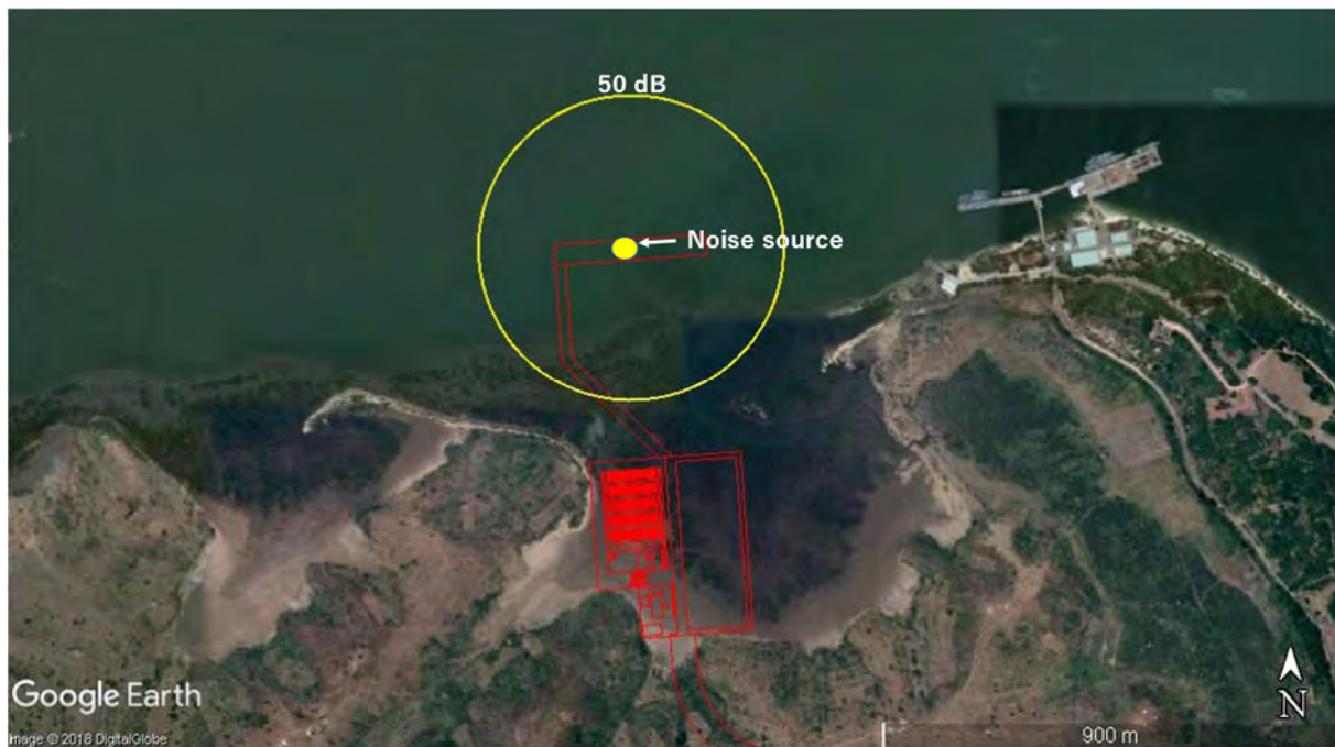
Figure 11.3.32 Predicted Noise Attenuation from Pile-Driving Works
