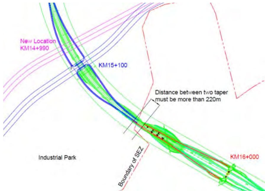
Figure 8.4.7 Problem of Distance between two Intersections
