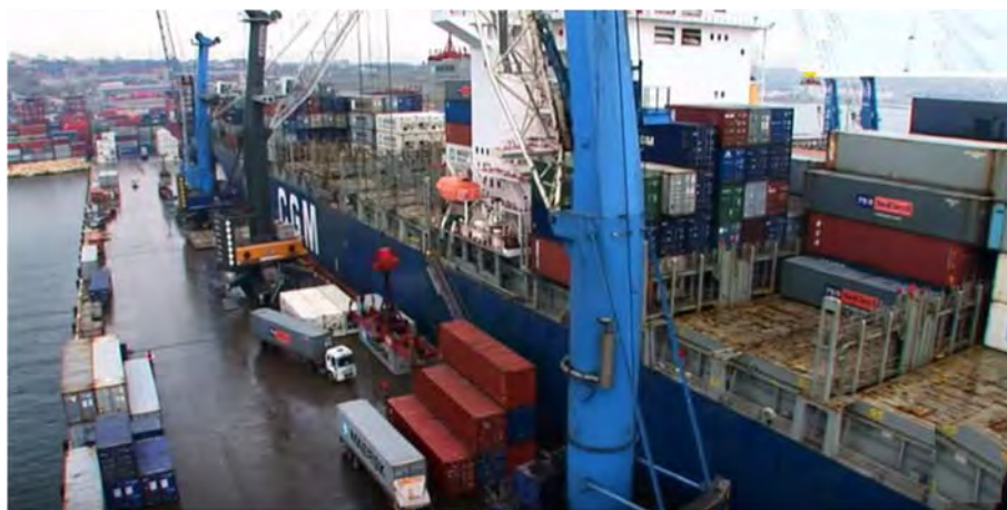
Figure 8.3.54 Quayside MHC Operation in Narrow Working Space on the Jetty (Berth width: about 35m)
