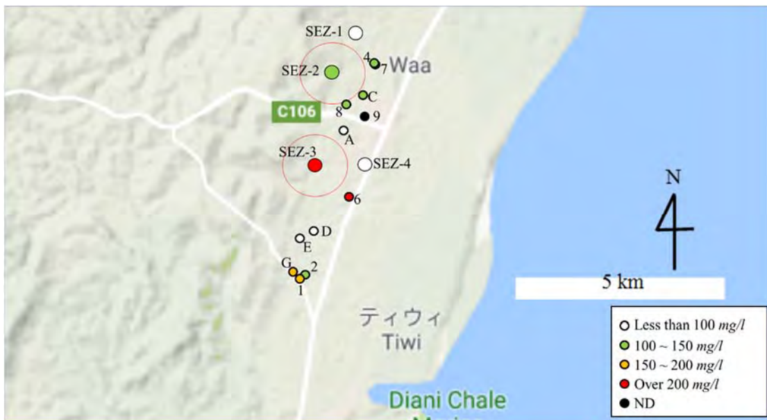
Figure 8.5.17 Location of Existing Boreholes and Chloride Ion Concentration
