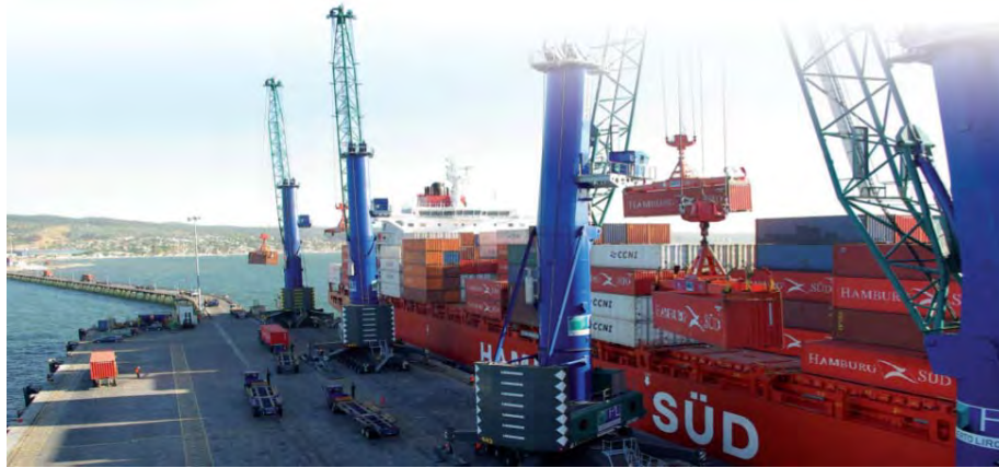
Figure 8.3.52 Quayside MHC Operation with Sufficient Working Space on the Jetty (Jetty width: about 50m)
