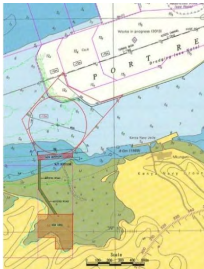
Figure 5.4.4 Dredging Area for New Navigation Channel and Basin (-13m)
