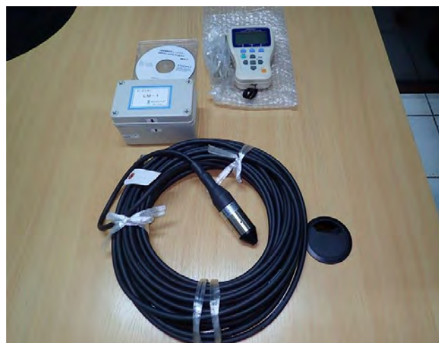
Water level sensor, data logger and data collector (at office of JICA Expert Team, 2018/02/26)
