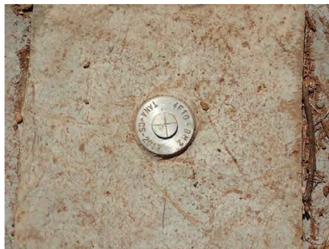
Bench mark for river cross section survey (4F10, 2017/09/27)
