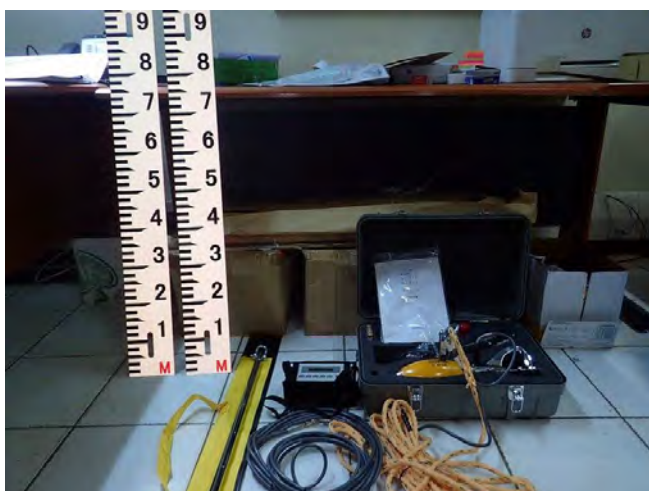
Staff gauge and propeller-type current meter with rods) (at office of JICA Expert Team, 2018/02/26)
