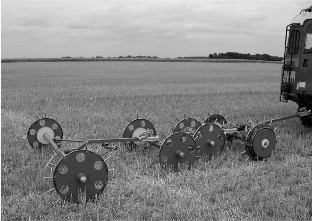
Fig. 5. Multidepth Continuous Electrical Profiling (MUCEP).
