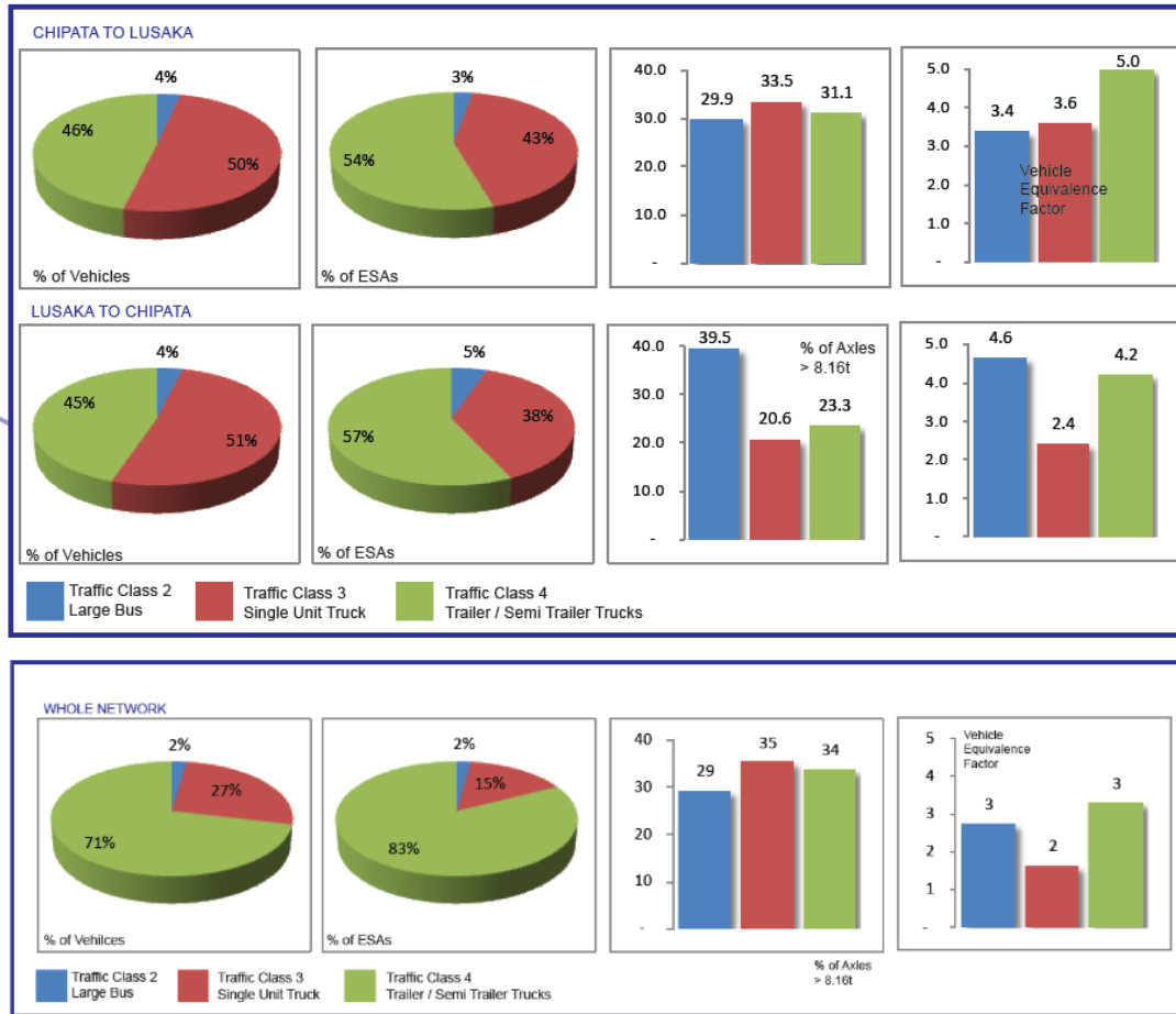
Figure 6.1-3 Characteristics of traffic on the Nacala Corridor
