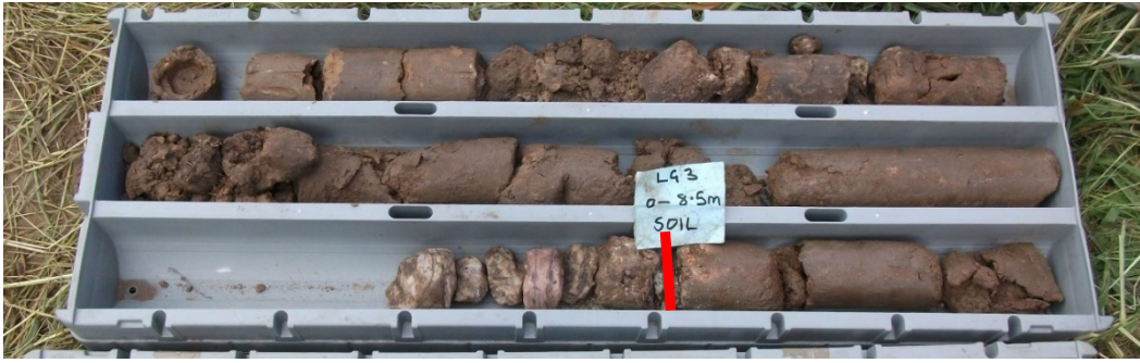
Photo 5.1-14 (BH-3) Boring core (fine sand and silty sand, weathered gneiss occurring along cracks at depths of GL-8.5 m or more)
