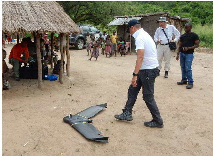
Photo EP.1-1 Fixed Wings UAV
