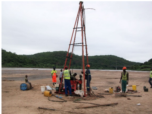
Photo 5.1-10 Boring survey at BH-2 (mid-channel)
