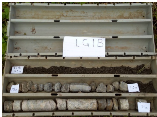
Photo 5.1-13 Cores taken at BH-1' (right bank)
