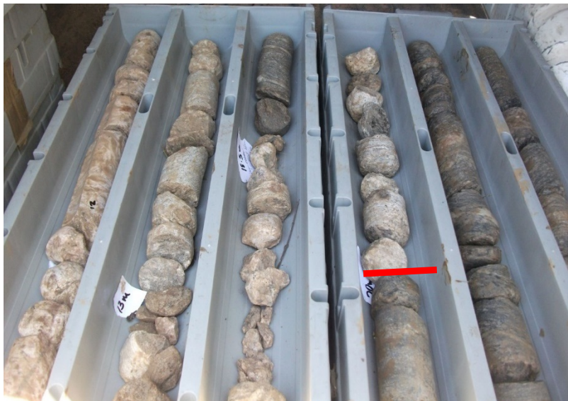
Photo 5.1-15 (BH-3) Boring core (gneiss, cracky hard rock at depths down to GL-20.0 m, hard rock at depths greater than GL-20.0 m)
