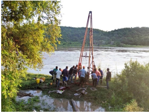
Photo 5.1-8 Boring survey at BH-1 (right bank)
