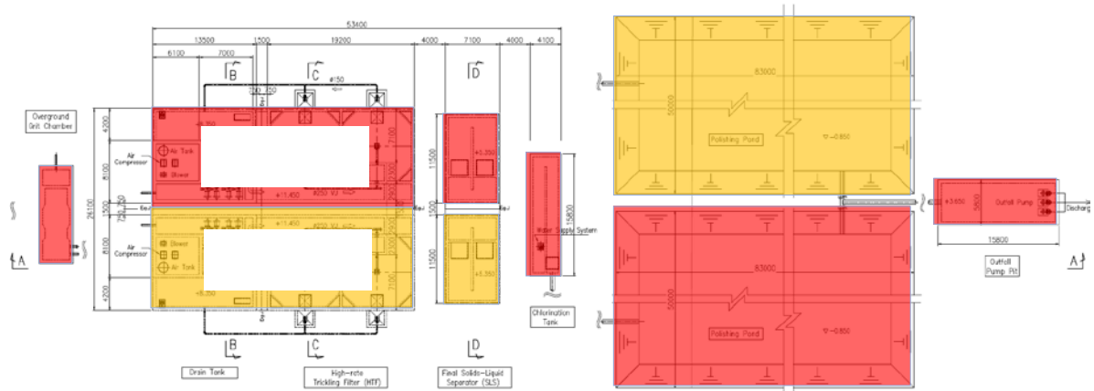
Figure 5.3-11 Stepwise Construction Plan of the Wastewater Treatment Plant
