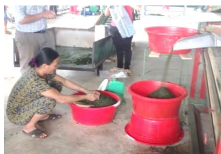
Processing line for sieving Tencha
