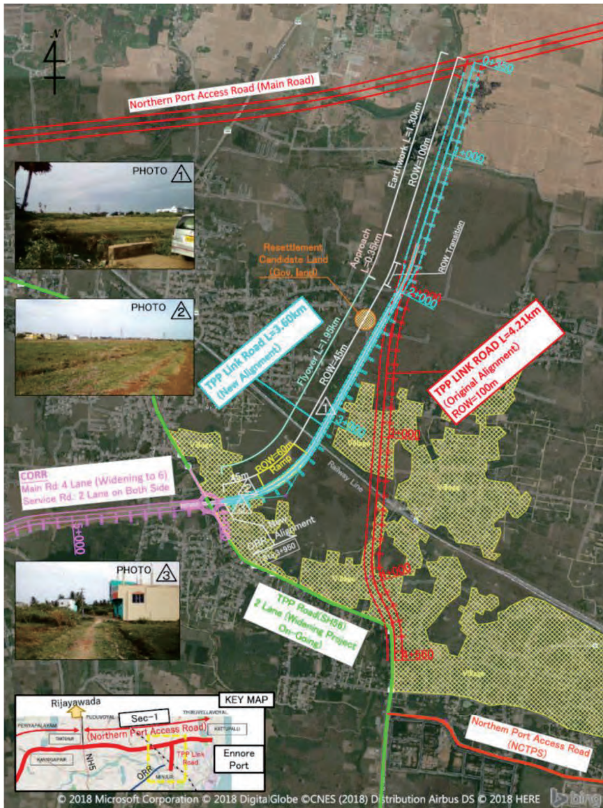
Figure 6.5.9 Alignment Change Plan of TPP Link Road
