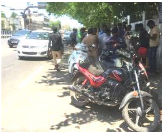
Figure 2.1.23 Reduction of Lane due to Sidewalk Stalls
