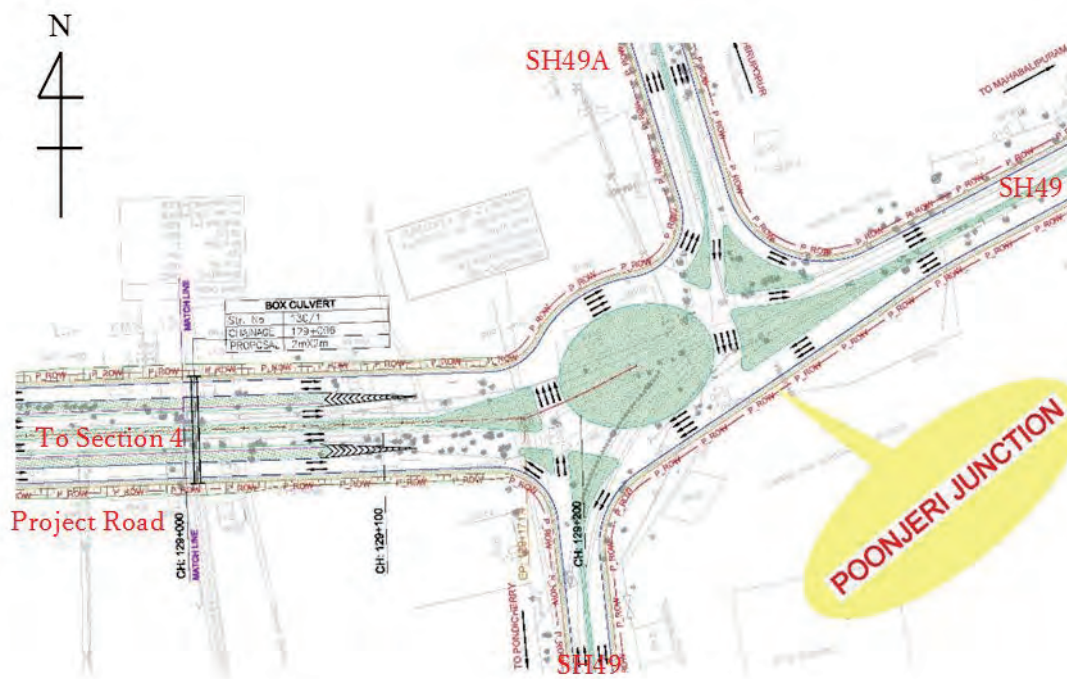
Figure 6.2.10 Plan of the Present Design of End Point
