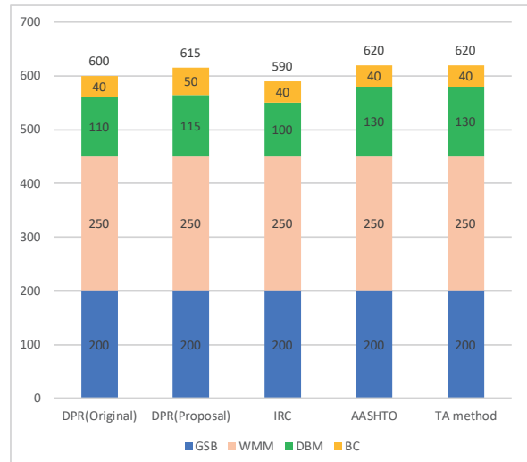
Pavement Thickness of Section 2 (Case 1)
