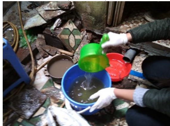
Photo 2-9 Sampling situation of wastewater from septic tank (HN2TR1)
