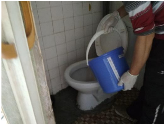
Photo 2-6 Inflowing situation of wastewater into septic tank (HN2TR1)
