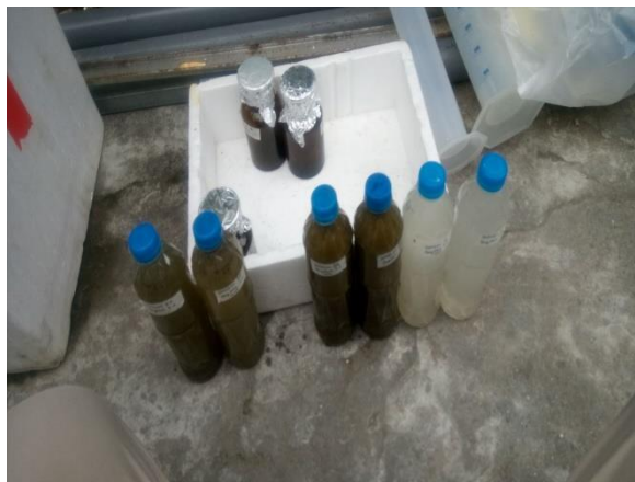
Samples: Greywater (right side), Influent (Black water + greywater: center) Effluent from septic tank (left side)
