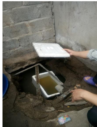
Sampling treated water from septic tank
