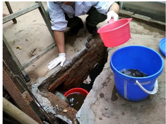
Photo 2-11 Sampling situation of wastewater from temporary toilet and septic tank (HN1HM1)
