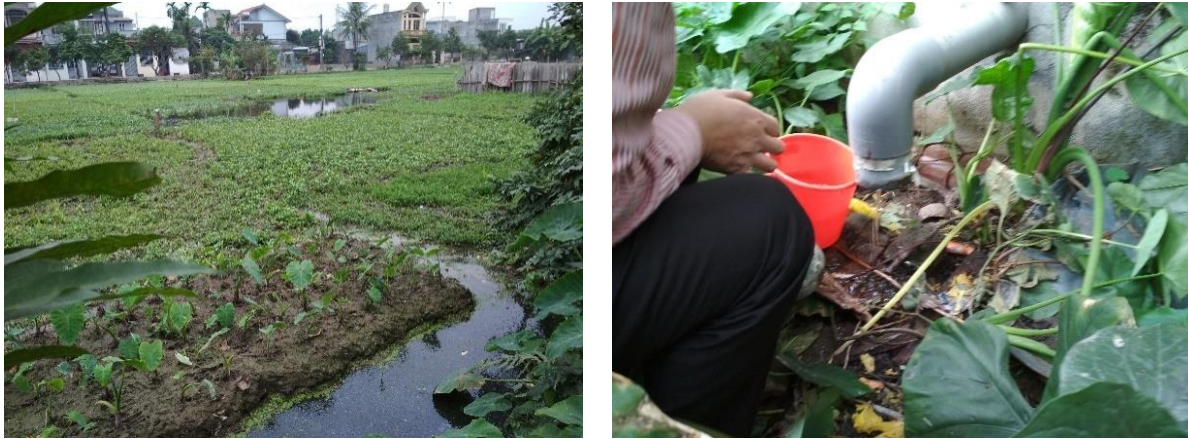
Photo 2-4 Photo Example of sampling of effluent from septic tank in Hai Phong (Independent house: 2018/1/20, treated water flows into wetland)
