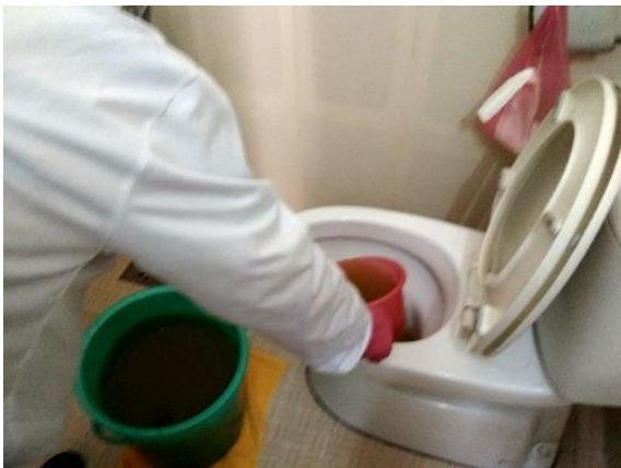
Photo 2-11 Sampling situation of wastewater from temporary toilet and septic tank (HN1HM1)
