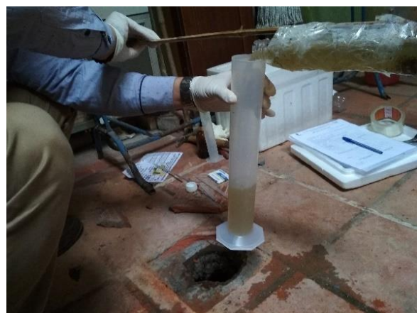
Photo 2-3 Photo Example of sampling of effluent from septic tank in Ha Noi(Independent house: 2018/1/16)
