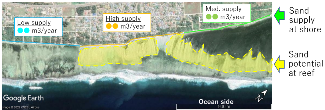
Figure 2.5.6 Example of Map for Sand Supply Volume and Sand Potential at Reef Flat
