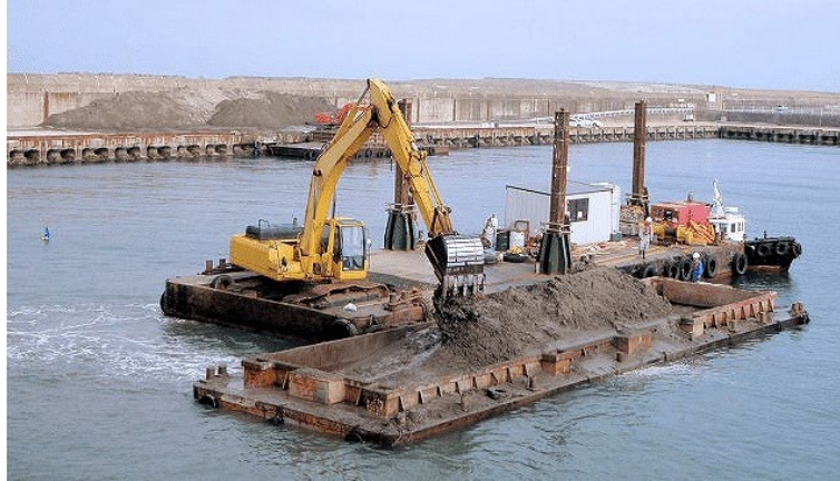
Figure 5.8.13 Example of an Excavation Dredger
