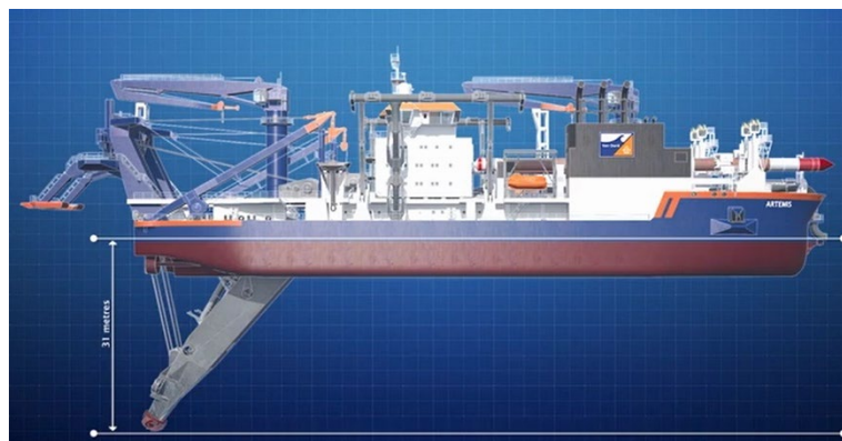
Figure 5.8.12 Example of a Cutter Suction Dredger
