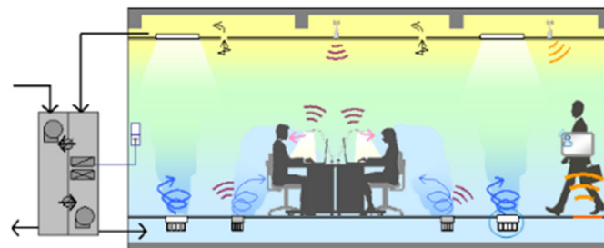
Figure 237 Task Ambient Air Conditioning System
