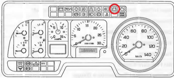
Generator warning light
