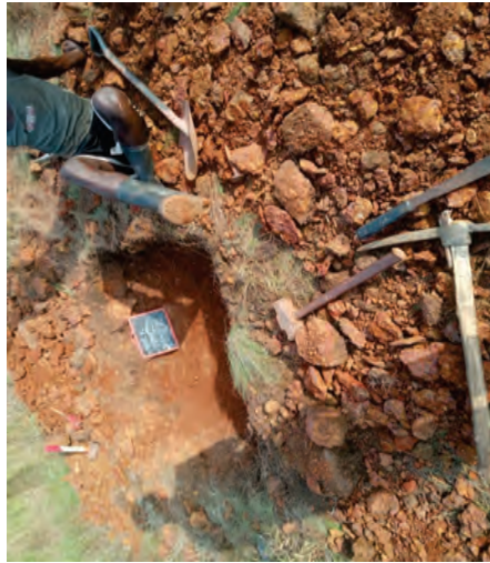
Figure 41: York Trial Pit-1 Terminated and Backfilled
