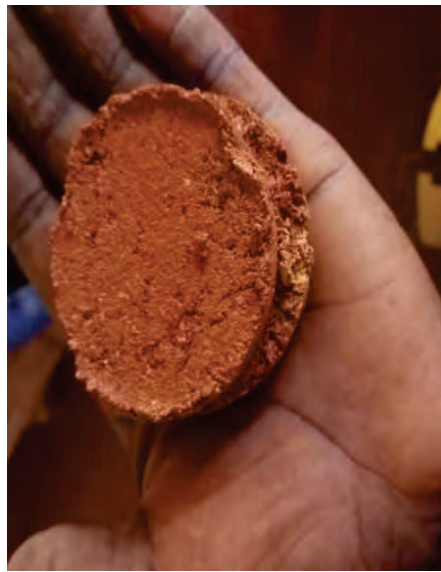
Figure 61: A Specimen in the Shear Box (Cylindrical shaped)
