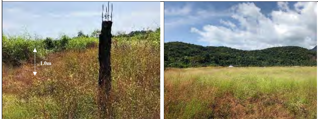
Photo A: The level difference between the front road and the site View from the project site to the road side. Since there is a 1.0m difference in level from the road. It's necessary an access road. Photo B: View of the project site The proposed construction site is relatively flat, but the surface is wet, so a 200 mm gravel bed will be considered.
