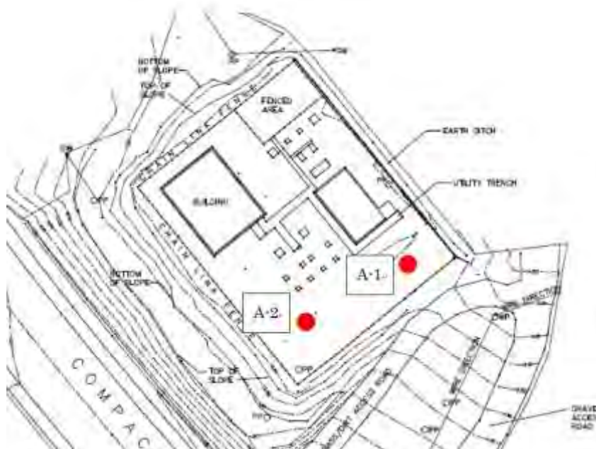
図 2.4.1 Investigation points at airai Substation
