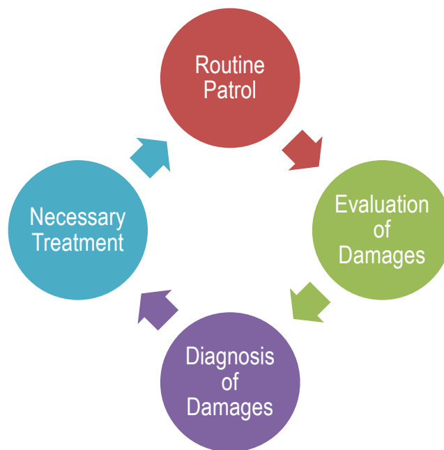
Figure 2.1 Maintenance Cycle of Routine Maintenance
