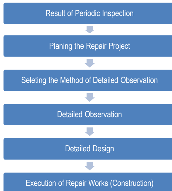
Figure 5.1 Procedure of Repair Works (Individual Bridge/Damage)
