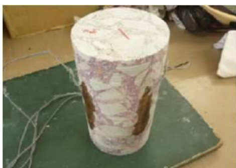
(Strain Gauge attached on the Side Surface of the Core Sample)
