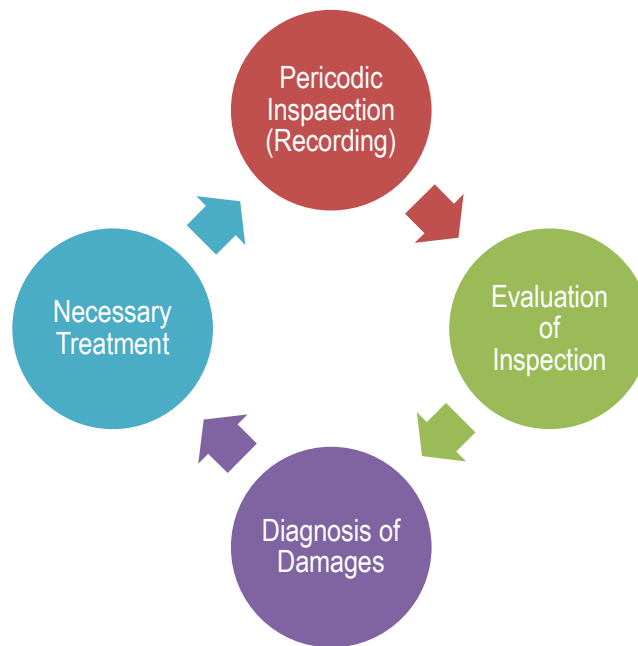
Figure 2.2 Maintenance Cycle of Periodic Maintenance
