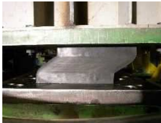
Figure 6.31 Example of Deformation of Aseismic Bearings
