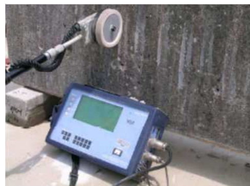
Figure 5.18 Example of Spontaneous Electric Potential Method
