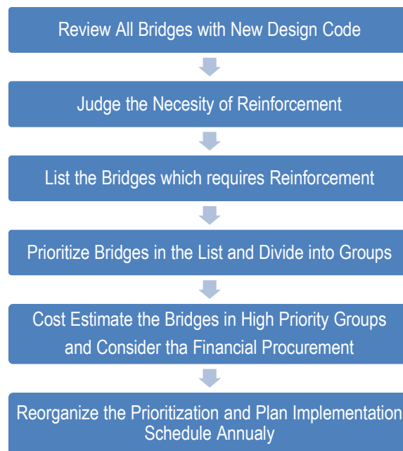
Figure 6.1 Procedure of Mid-term Strengthening Plan
