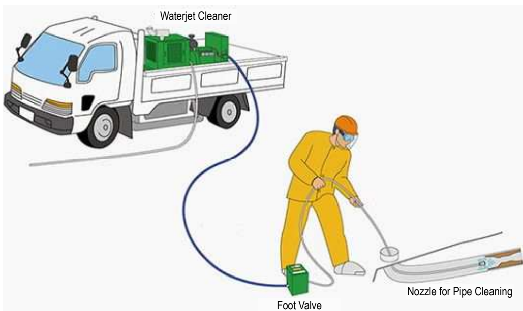
Figure 4.3 Example of Cleaning Drainage Pipes by Waterjet Cleaner
