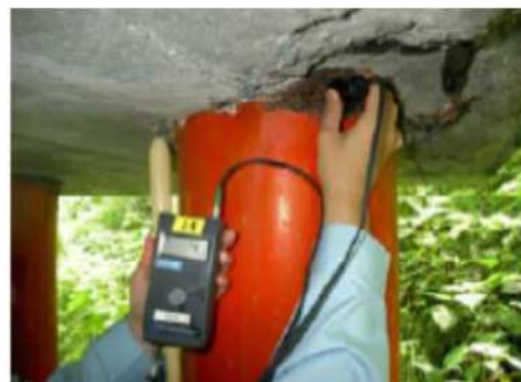
(Indirect Measurement by Ultrasonic Wave)
