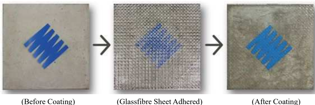
Figure 5.33 Examples of Skelton Coating of RCC Members
