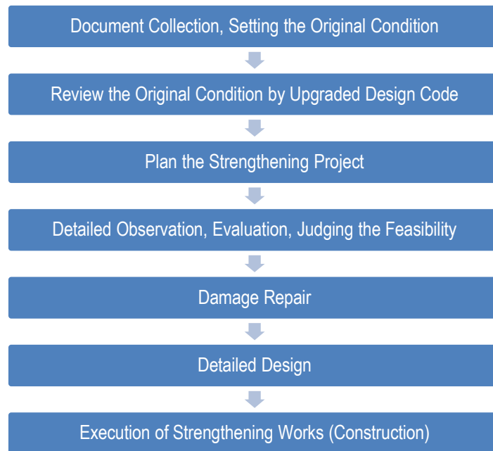
Figure 6.2 Procedure of Strengthening Works (Individual Bridge)
