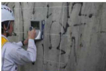
Figure 5.15 Examples of Electromagnetic Wave Radar Method
