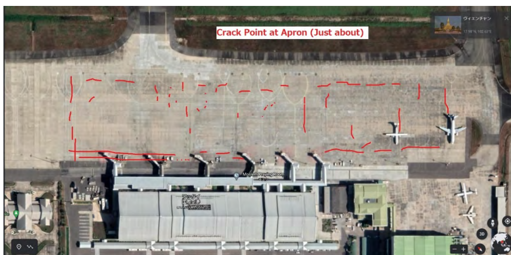
Figure 4.22 Location of Cracks in International Apron
