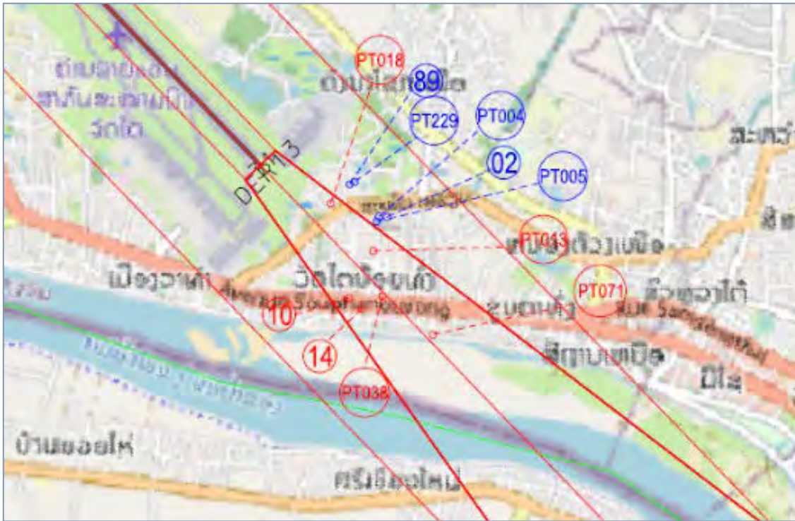
Figure 4.38 OLS Assessment Results: (2) Instrument Approach Runway (300 m)
