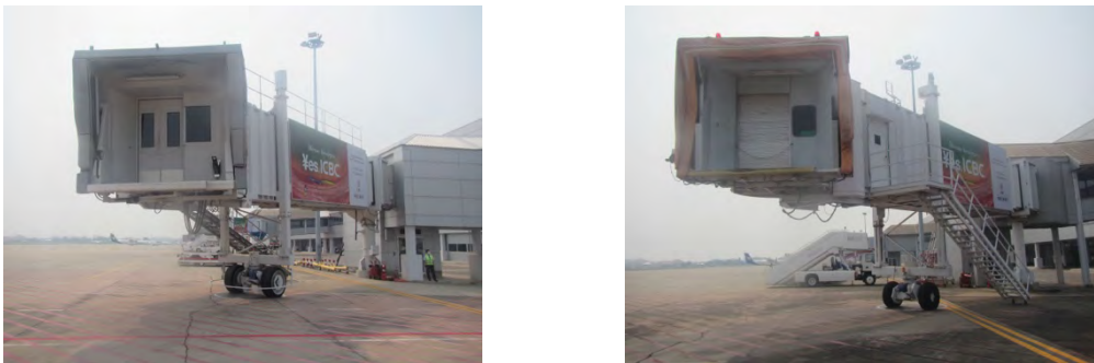
Figure 2.67 Passenger Boarding Bridge (left: Shinmaywa, right: Bukaka)
