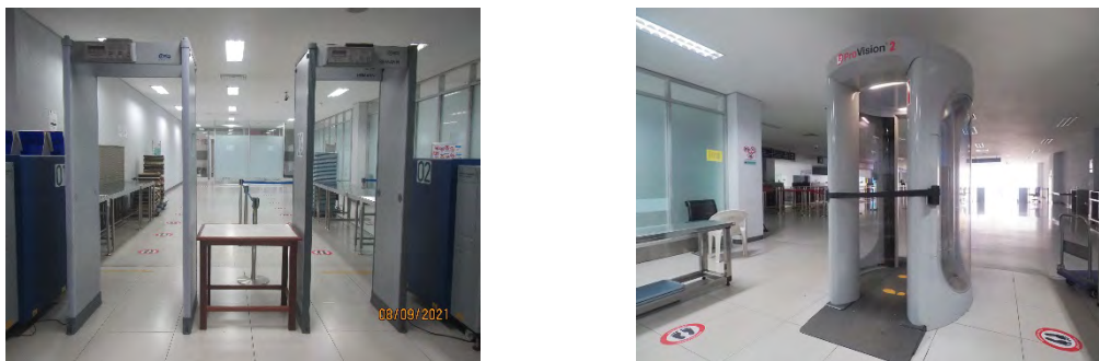
Figure 2.66 Walkthrough Metal Detector (left) and Full Body Scanner (right)
