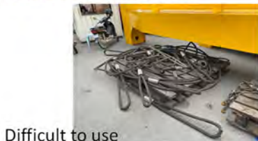
Difficult to use Risk of entrapment
