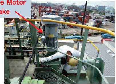
Clearance of Brake Pad of Traverse Motor is checked and Brake unit is cleaned by air-brush.
