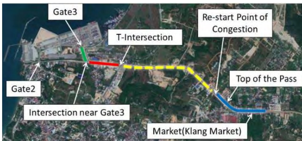
Waiting Queue of Trailers from the Gate-3 to the Outside (Colored by Area)
