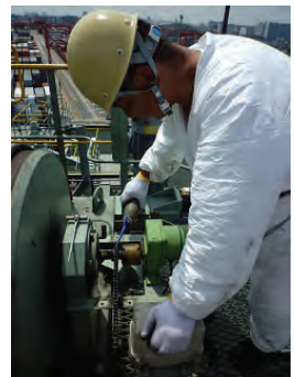
Confirmation of Cam type limit switch and
