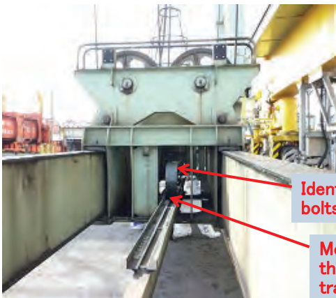
Refueling of grease to Sheave bearing
