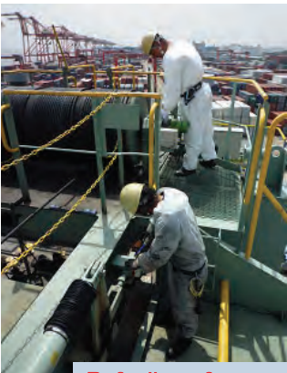
Refueling of grease to Link pins and Pin of Rope End Socket of Anti-sway
