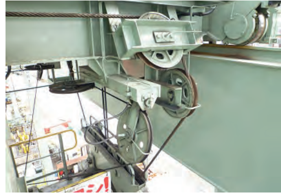
Refueling of grease to Sheave bearings for Anti-sway and Main Hoist
