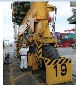
Lubrication to Pins of Steering Power Cylinder
