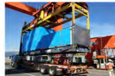
Lock/unlock is done by the rope. The hydraulic type is also available
