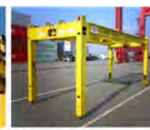
Attachment used in Kobe Terminal. Less vibration, up to 2 meters over height.
