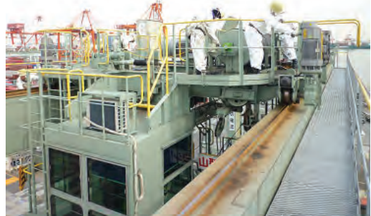
Refueling of grease to Bearing of Drum Shaft and drive chain, etc.
