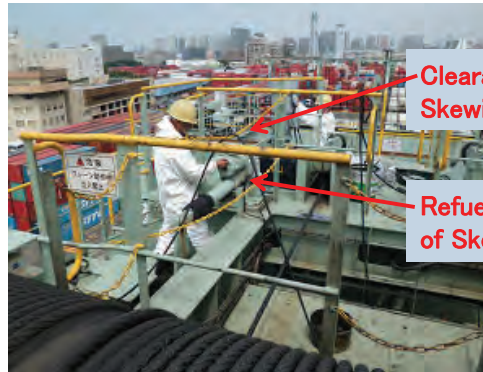
Clearance of Brake Pad of Traverse Motor is checked and Brake unit is cleaned by air-brush.
