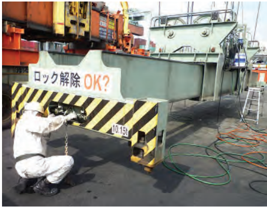
Moving parts and their guide/Guide tray are cleaned by air-brush
