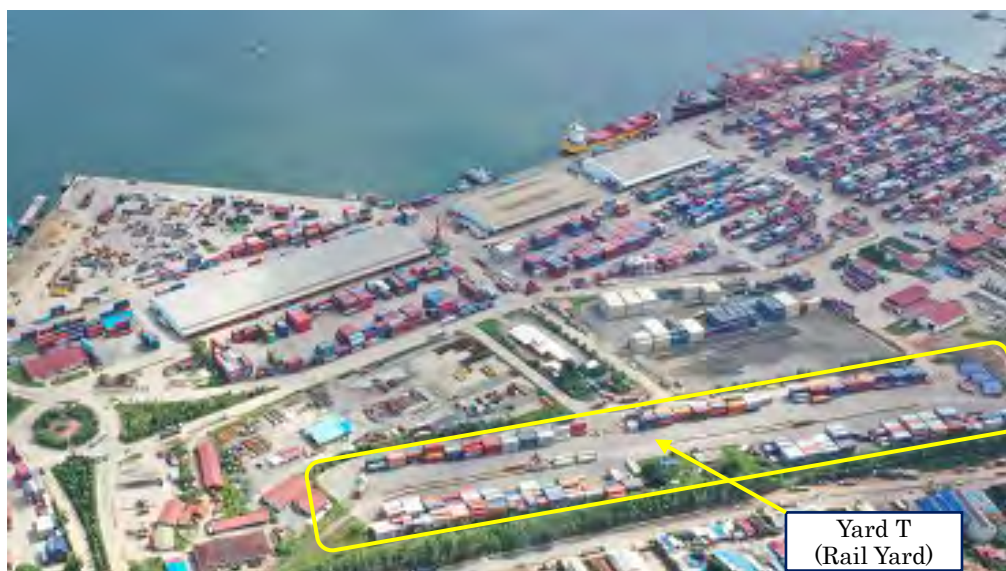
Figure 2.3-1 Positional relationship between CY and Rail Yard
