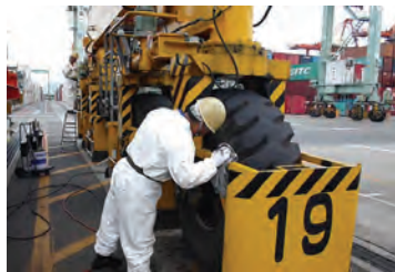
Wear of Gantry Tyre is checked.
