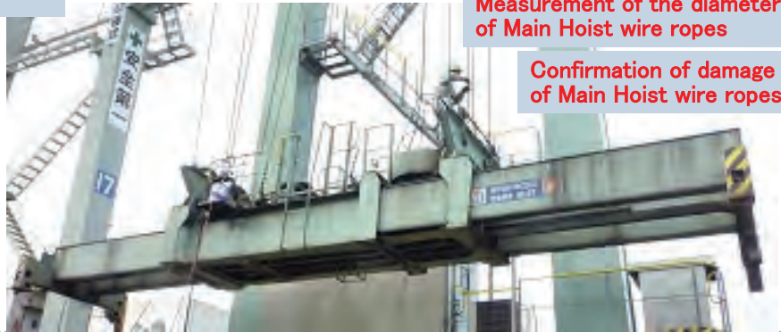
Confirmation of the movement of the Twist-lock Cylinder
