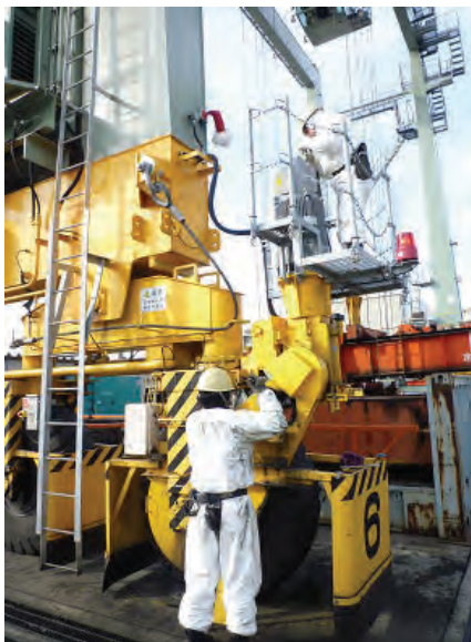
Adjustment of tension of Gantry Drive Chain and Refueling of grease to Drive Chain
