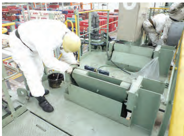
Refueling of grease to Bearing and Pins of Main Hoist Fleet Sheave
