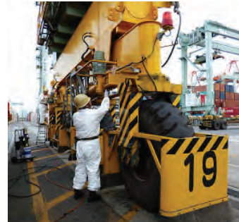
Lubrication to Pins of Steering Power Cylinder
