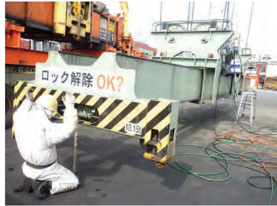
Confirmation of the movement of the Twist-lock Cylinder
