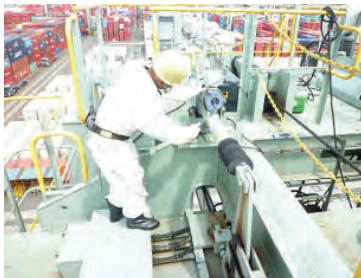
Refueling of grease to Pins of Power Cylinder for Spreader Skewing
