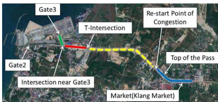
Figure 6-4 Traffic congestion from the gate to the outside of the port (areas classified by color)
