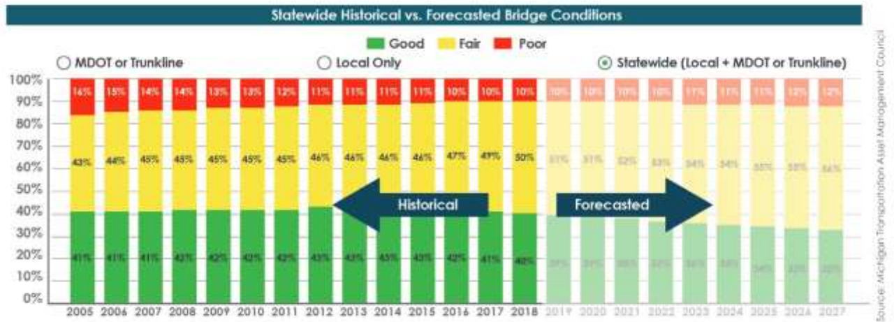
Figure 19. Example website dashboard showing an analysis for bridge conditions.
