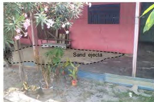
Fig. 11. Sand ejecta found at the upper part outside of flow area (Balaroa).
