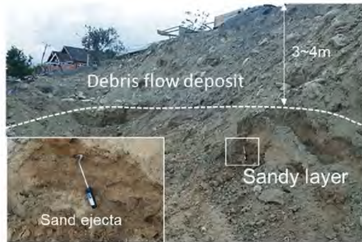
Fig. 8. Soil profile observed at the main scarp of flow-slide in Balaroa.
