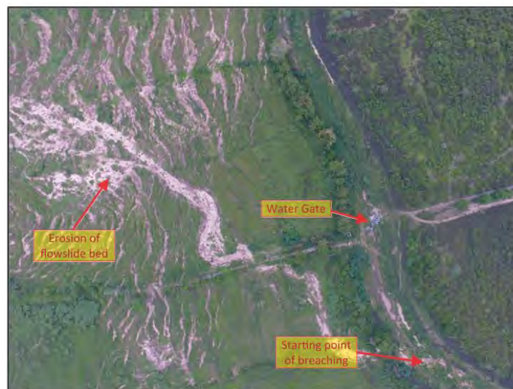
Fig. 11. UAV imagery of channel breaching and water gate destruction in Jono Oge (Location No. 1 of Fig. 10).
