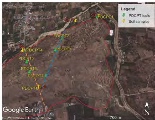
Fig. 13. Locations of the PDCPT and collected soil samples at Jono-Oge.
