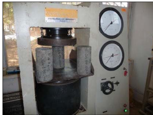
Compressive Strength Test
