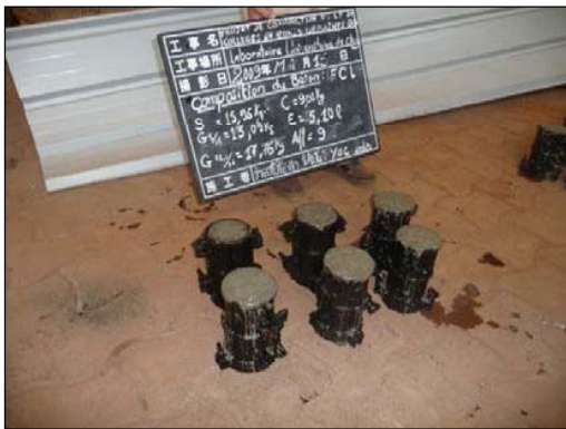
Test Piece Sampling for Compressive Strength
