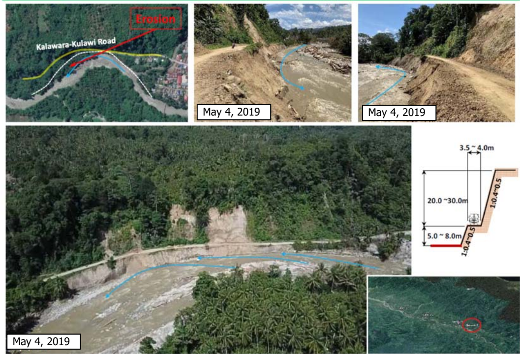
Figure 3-32 Landslide condition at Landslide-4 in Gumbasa –Saula Area
