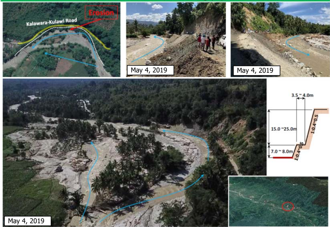
Figure 3-31 Landslide condition at Landslide-3 in Gumbasa –Saula Area
