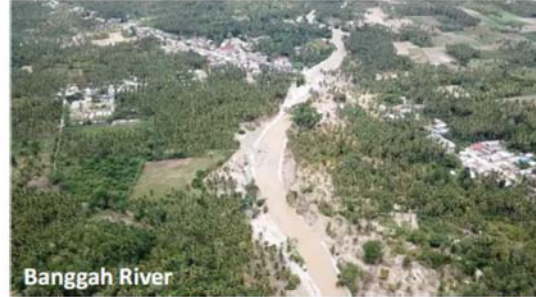
The unstable sediment generated by the slope failure in the mountainous area and the sediment flow generated by the flood caused a flood.
