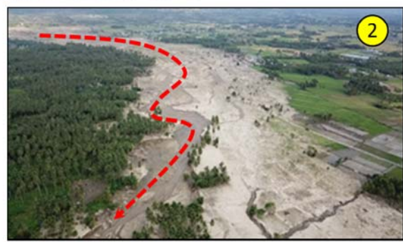
Flash flood inundated area from liquefaction-landslide area of Jono Oge
