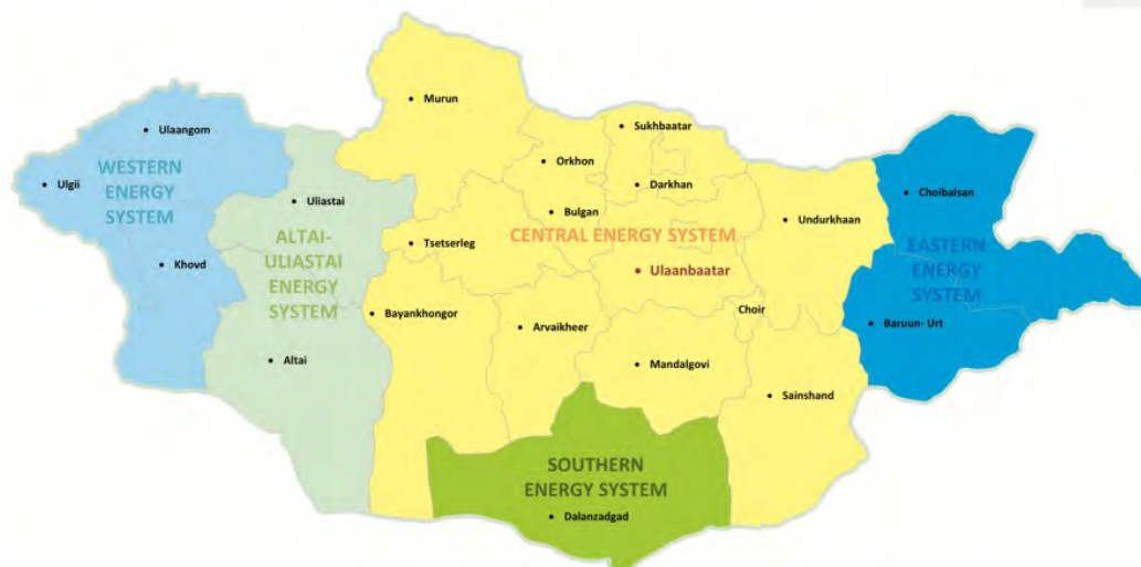
The Energy Sector of Mongolia consists of five independent electric power systems. (WES, AUES, CES, SES, EES)
