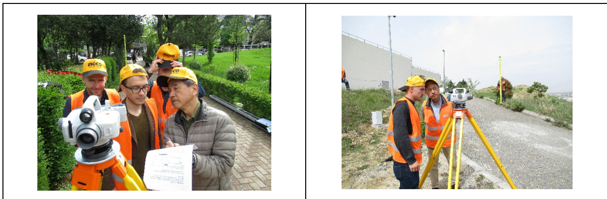
Photo 4-2 (Left) Inspection and adjustment methods of level, (Right) First order leveling Observation
