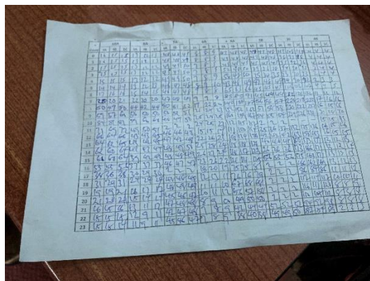
Figure 5-4.10 11kV feeder load current recording
