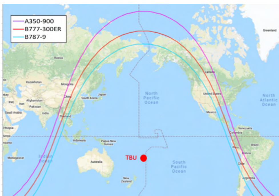
Figure 4-3-1 Flight Range from TBU by Selected Aircraft with Full Passenger Payload
