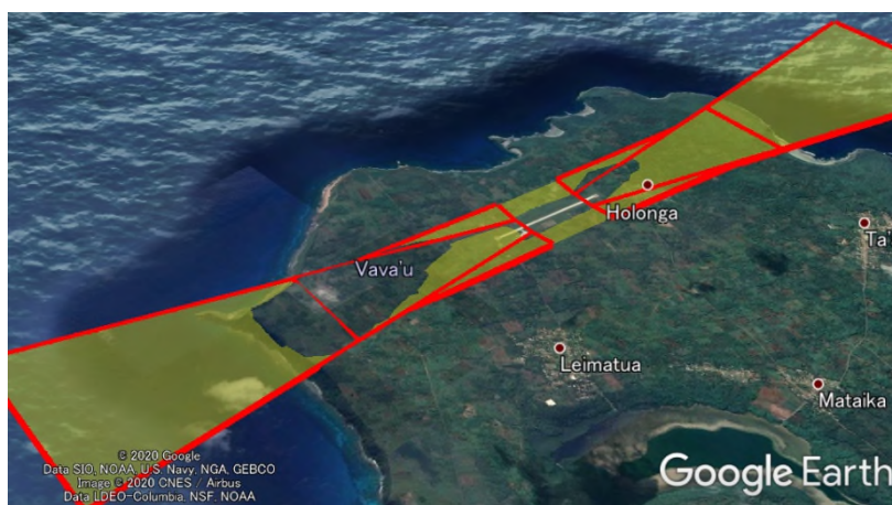
Figure 5-2-7 Perspective of OLS at VAV
