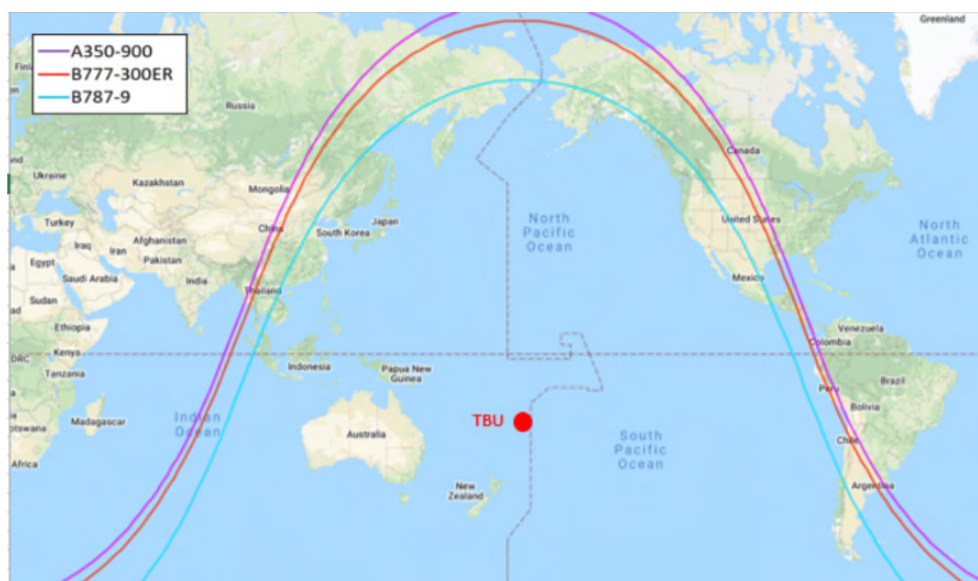
Figure 4-3-2 Flight Range from TBU by Selected Aircraft with ACN ≤ 77
