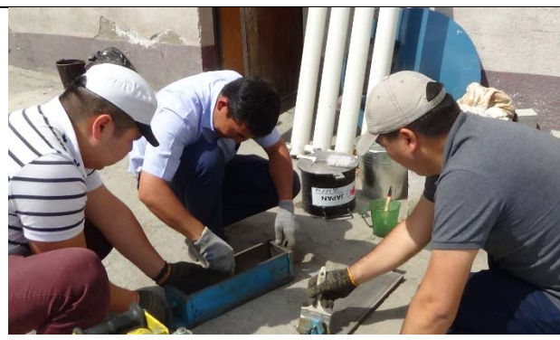
Photo 4: Preparation of molds for bending test.
