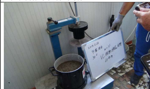
Photo 3: Testing on VC device.
