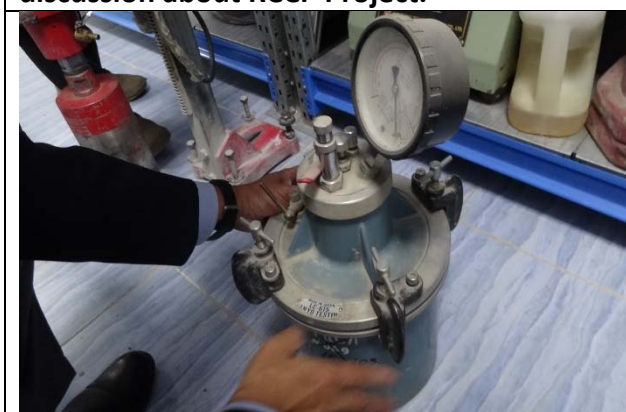
Photo 3: Device for air measuring in the fresh concrete mix.
