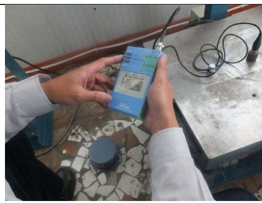
Photo №4: Inspection vibration plate of VC device
