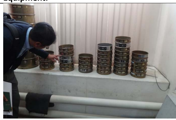
Photo 4: Sieve for determining size of gravel and sand.
