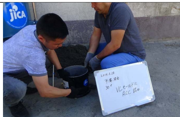
Photo 2: Mr. Tursunbek fills the tank with fresh concrete mix.
