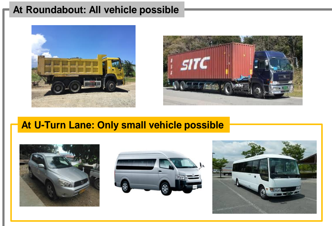
Figure 2.19 Design Vehicle at U-turn Lane and Roundabout
