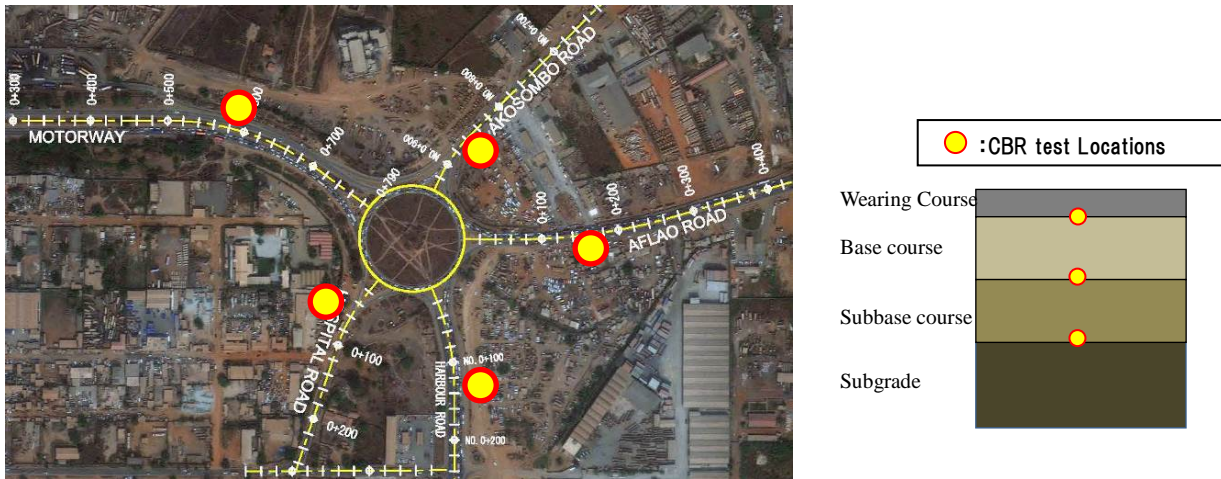
Figure 2.2.2-28 Existing Pavement Survey by Soil Compaction Tester
