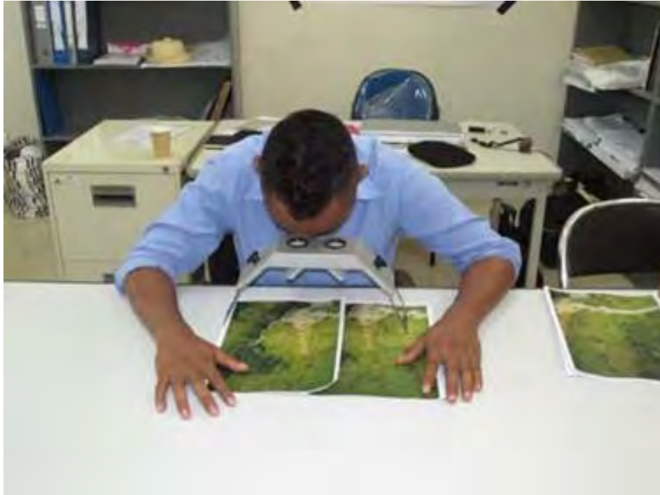
Figure 12 — Stereoscopic viewing of a pair of aerial photographs
