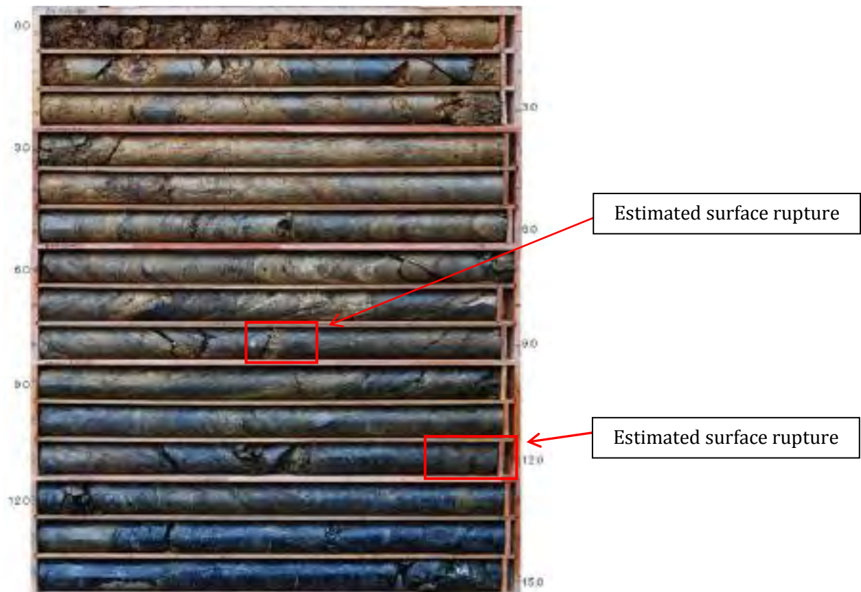
Figure 19 — Sample of undisturbed core sample in mass movement
