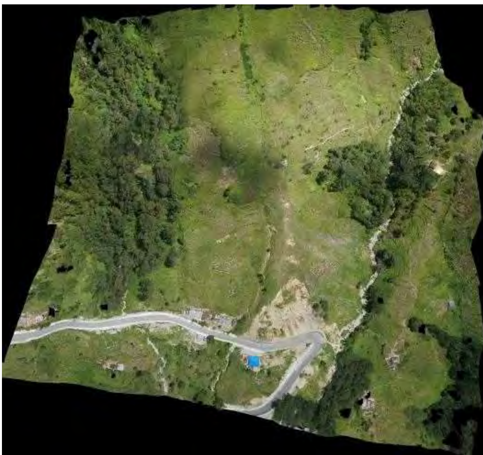
Figure. 12 The Example of Output (Ortho Photo)
