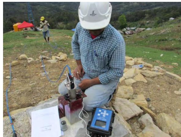
Figure 22 — Reading of values of inclination of the probe with the logger
