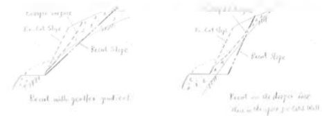
Figure 9.3 Two ways for recut
