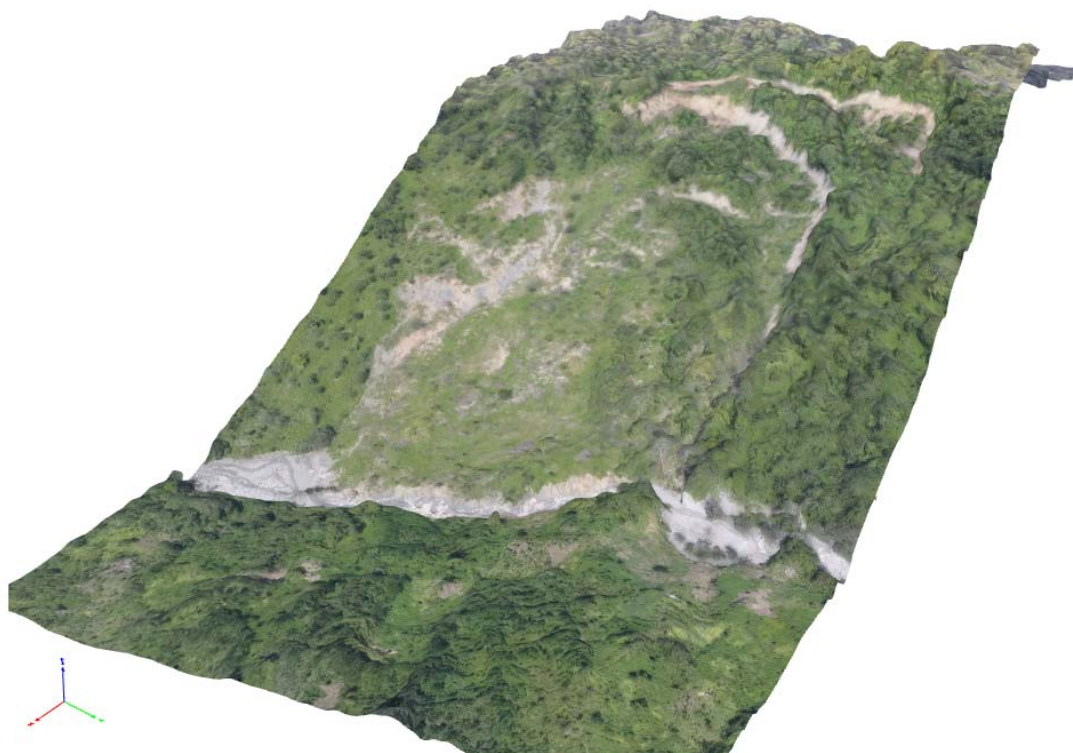
Figure 2.17 3D topographic model produced from UAV survey results
