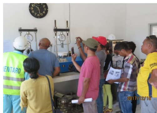
Marshall test during asphalt pavement workshop 2 (15 December, 2017)
