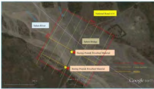
Figure 2.2 Location of Geotechnical and Topographic Survey
