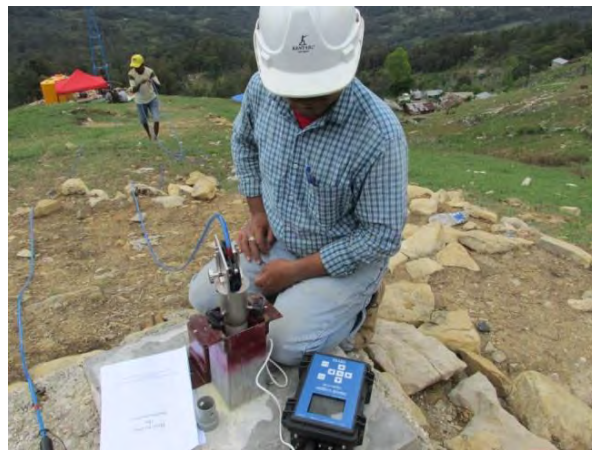
Figura 22 — Lee kona ba valor husi inklinaun husi sonda ho logger
