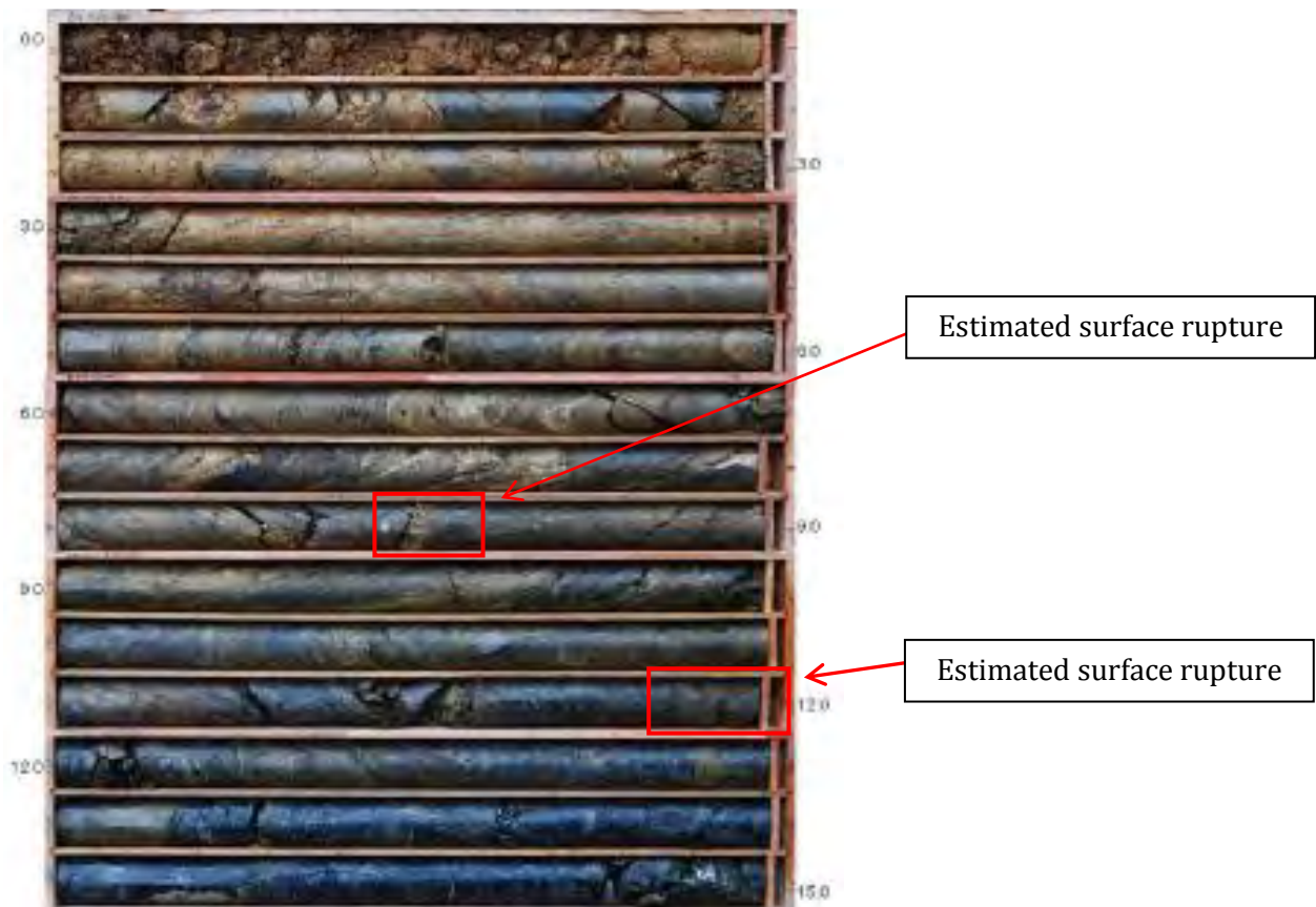
Figure 19 — Simple of undisturbed core sample in mass movement
