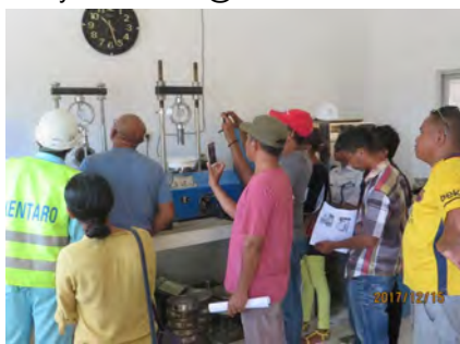
Work Shop 2: Marshall Stability Test , measuring Stability and Flow value at Laboratory @2017.12.15
