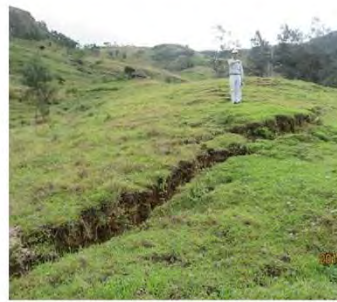
Scarp (long, steep slope) suspected of landslide
