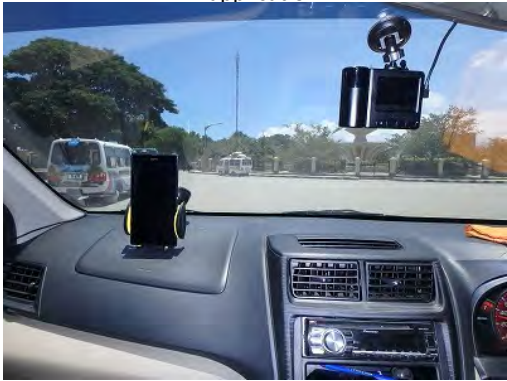
Data collection by Drive Recorder and IRI smartphone application
