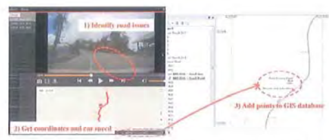
Example of data input from the video of a dashboard camera to the GIS database
