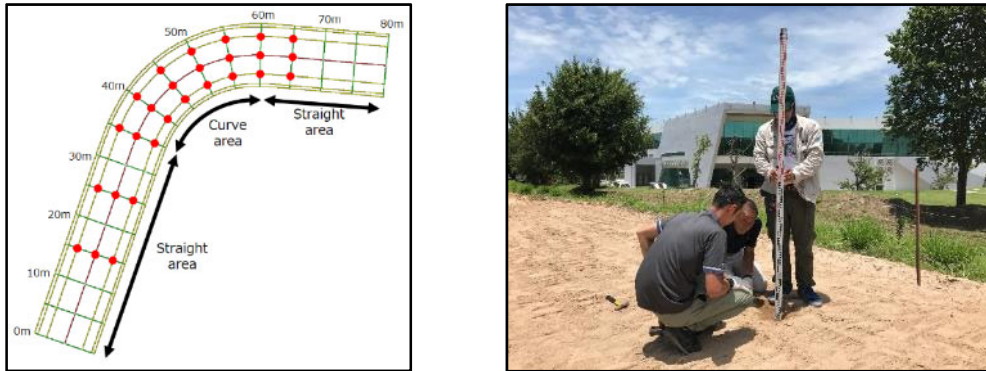
Fig. 49 Left: Position of Height Piles, Right: Height Adjustment Work
