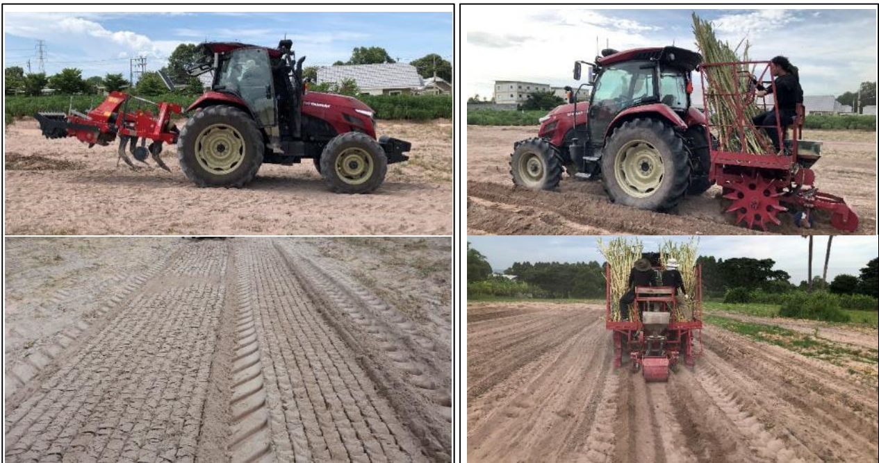
Fig.57 Top left: Mini combine, Bottom left: After work, Top right: Sugar Cane Planter, Bottom right: After work
