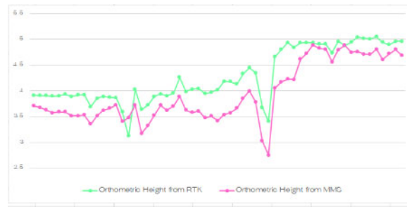
Fig. 10 Comparative ground elevation results by RTK (Green) and MMS (Red)
