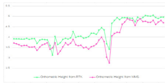
図 10 Comparative ground elevation results by RTK (Green) and MMS (Red)
