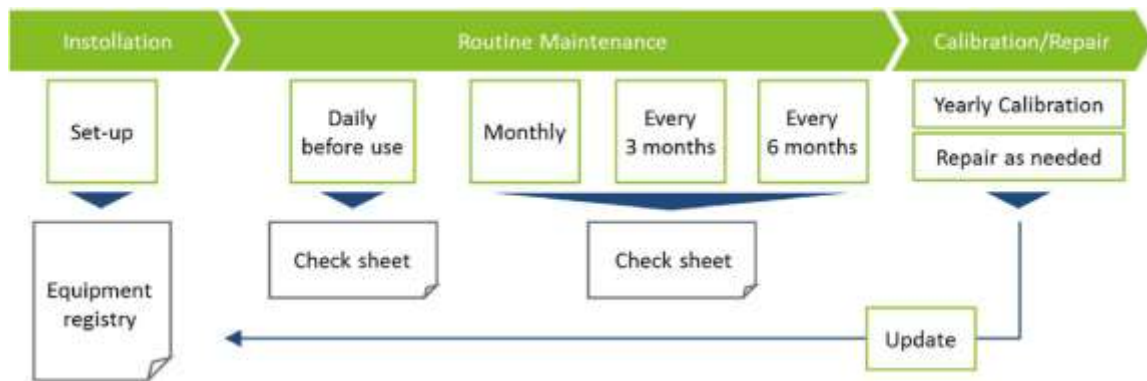
Figure 9 Overall picture of maintenance management of equipment in Japan
