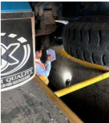
An inspector (CMVIC) who performs visual inspection using check sheet in pilot project
