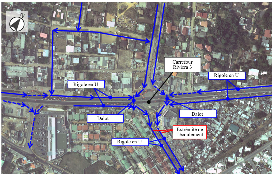
Figure 3.1.4 Carrefour Riviera 3 Situation des installations de drainage
