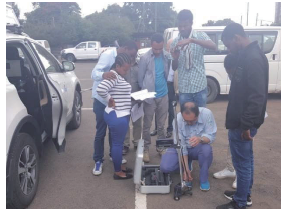
b) OJT on how to use Dip Stick for road roughness measurement
