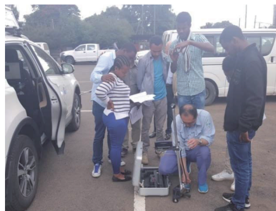
b) OJT on how to use Dip Stick for road roughness measurement
