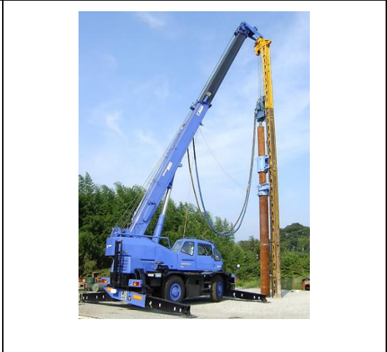
Figure 7.2-3 Boom Suspension Type
