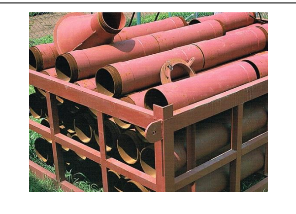
Figure 6.1-26 Screw Type Tremie Pipe
