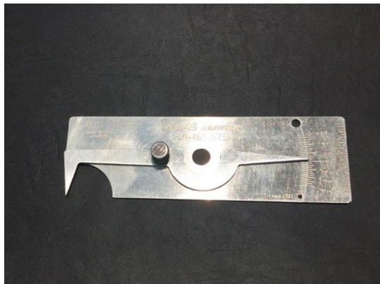
Figure 7.3-28 Welding Inspection Gauge
